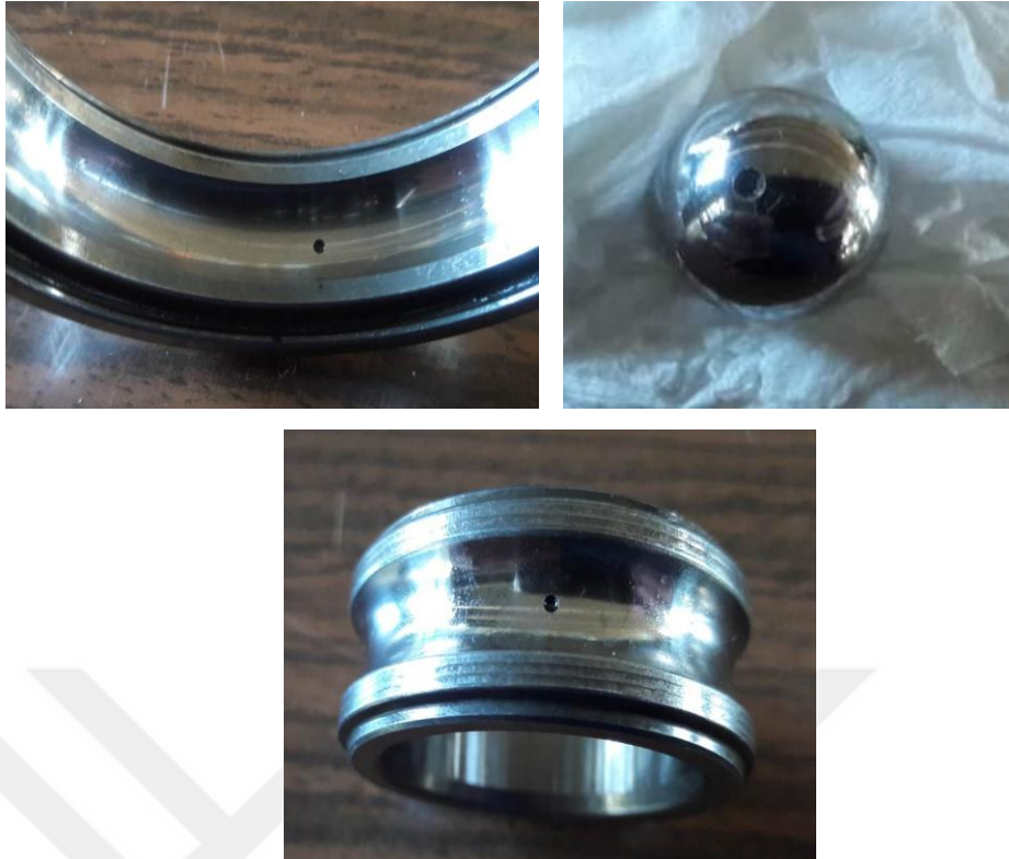
Figure 4.3 Artificial defects on the bearing components.
