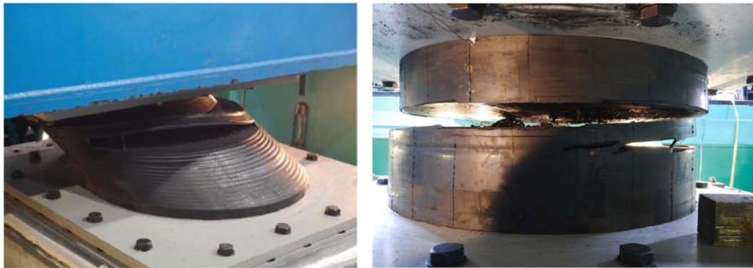
Figure 2.21 The views of the typical shear failures of LRB [98]
