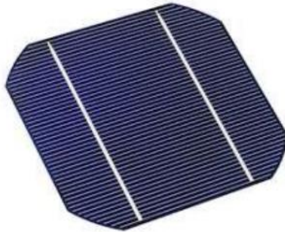
Figure 2.3. Monocrystalline silicon solar PV cell (Roy et al., 2014)
