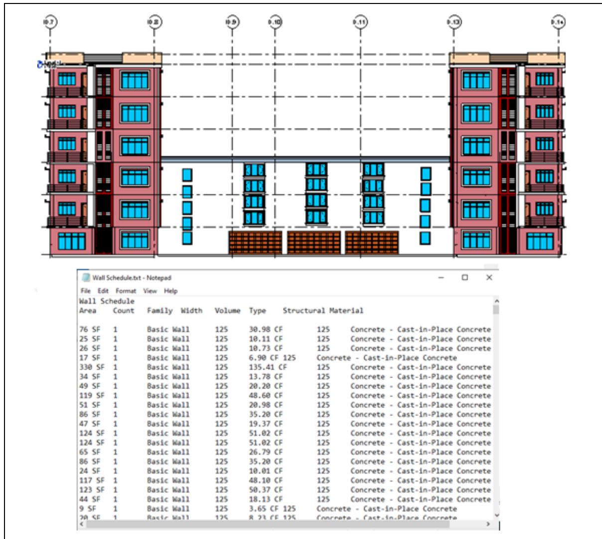
Figure 3.14: Calculate The Quantities of The Building.
