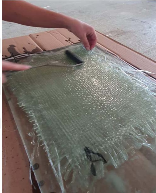
Figure 3.8. Removal of excess resin with a roller
