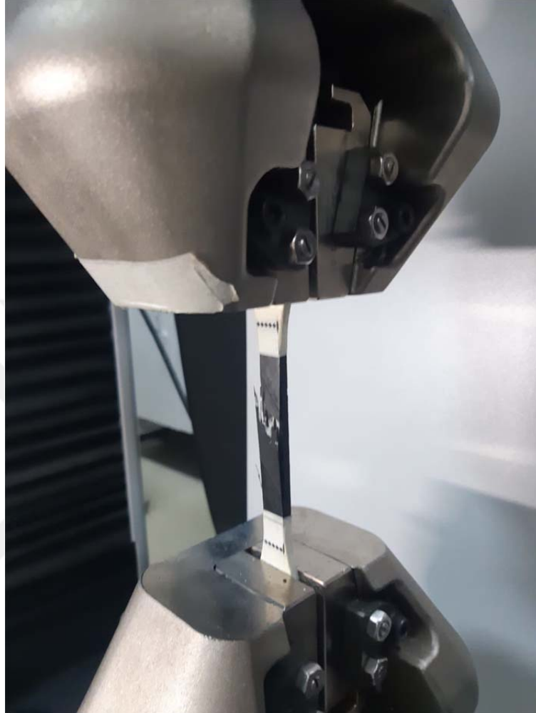
Figure 3.16. Moment of application in Tensile Testing Machine
