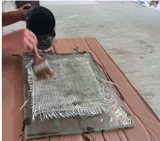
Figure 3.7. Applying resin between fiber layers
