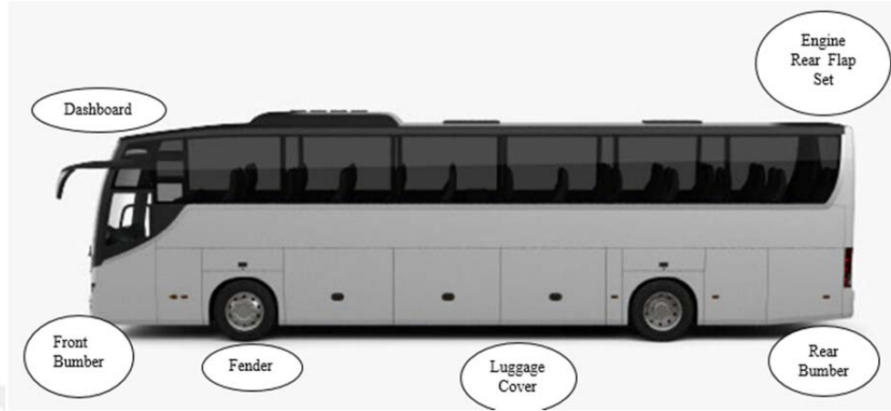
Figure 1.3. Major parts that composite materials can be applied on a bus
