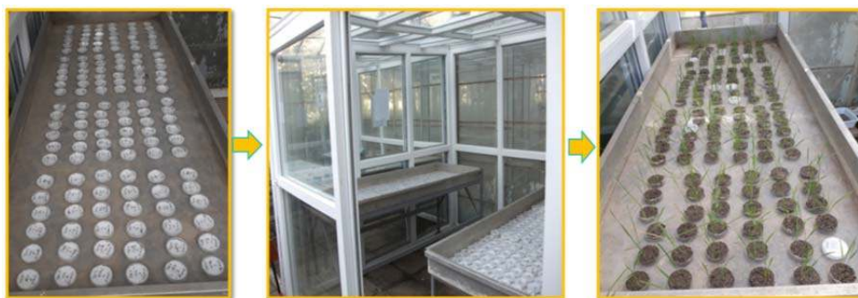
Figure 3.12. Filter paper-based seed germination test in daylight cabin.
