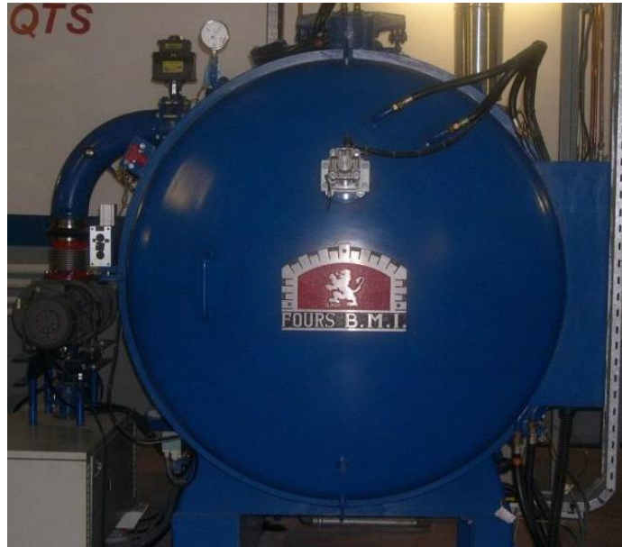
Figure 4.1 Image of the industrial vacuum furnace
