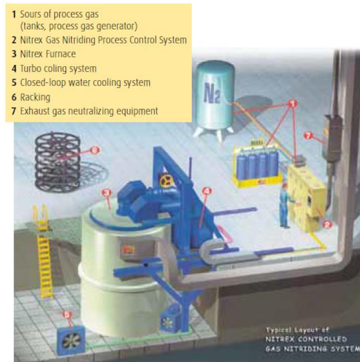
Figure 2.17 Pit-type furnace installation used for gas nitriding [32]
