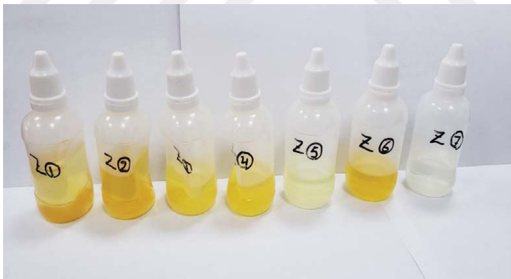
Figure 3.7. Solutions of crude oil samples after digestion by a closed MW system
