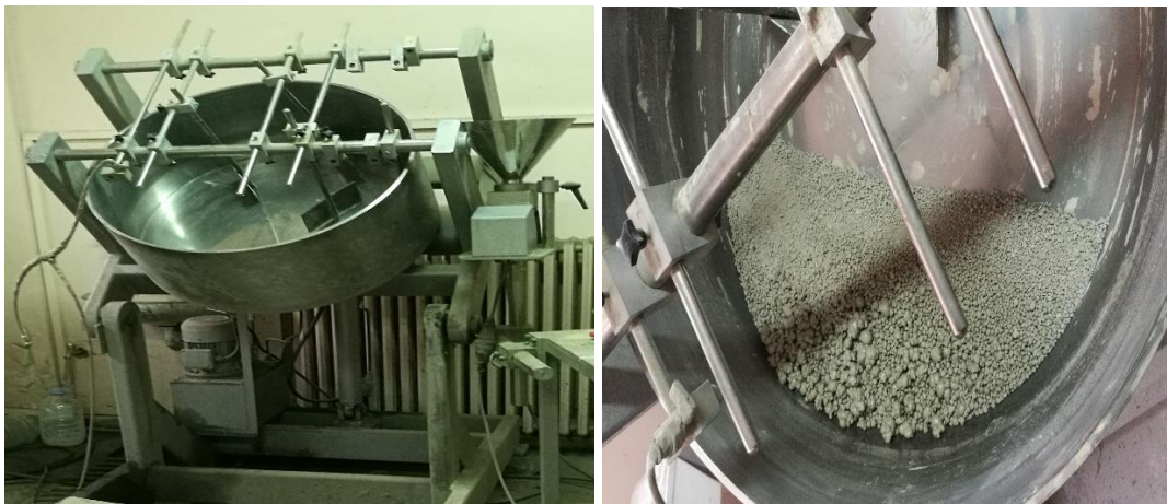
Figure 3.3 Disc pelletizer machine and geopolymerized stabilizer
