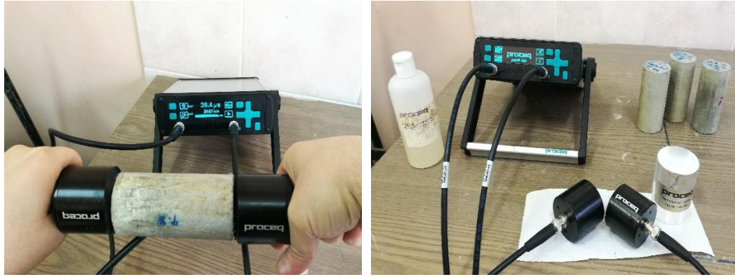
Figure 3.10 Ultrasonic pulse velocity test instrument and view of the test in progress
