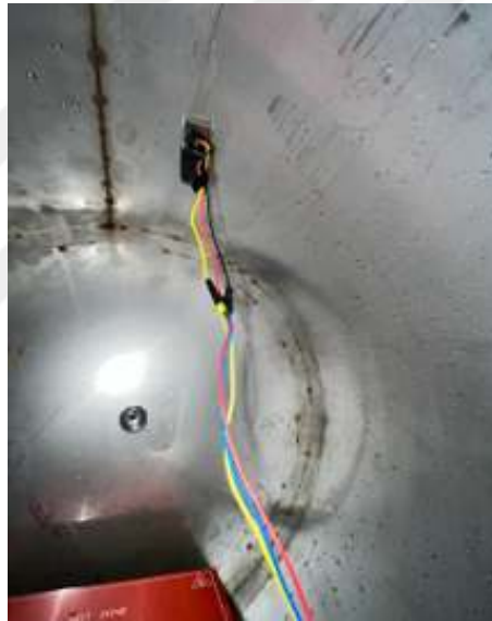
Figure 2.51: Water condensation on internal surface of drum
