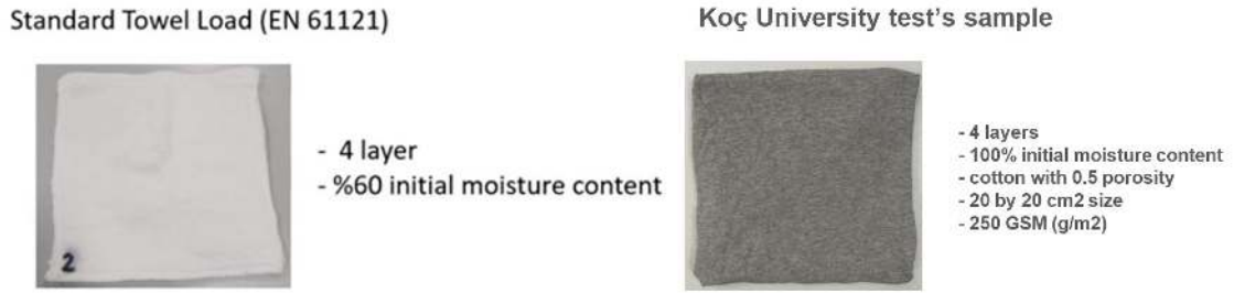
Figure 4.17: Sample prepared by Arçelik team for Çayirova tests and Koç University test's sample.
