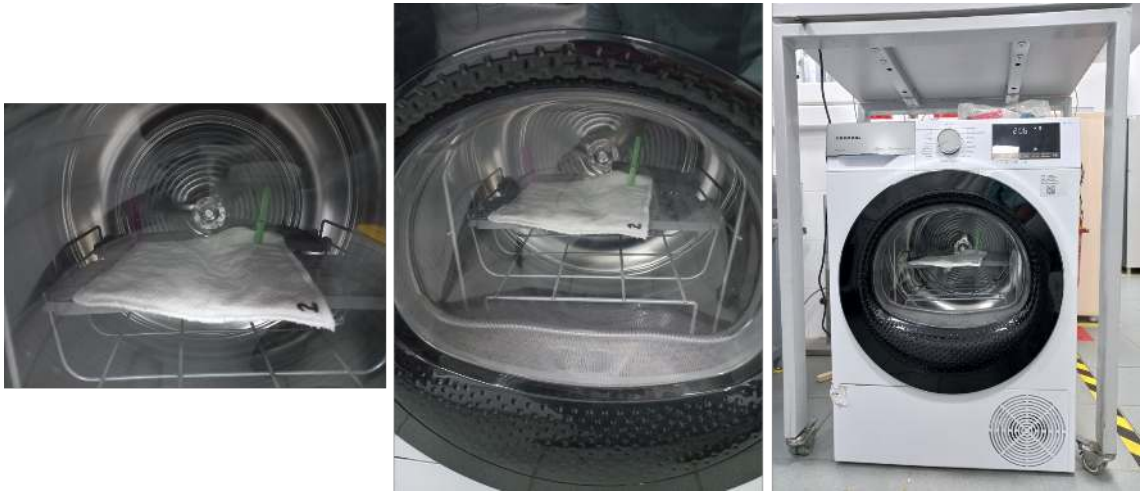
Figure 4.15: Arçelik hybrid HP dryer test setup
