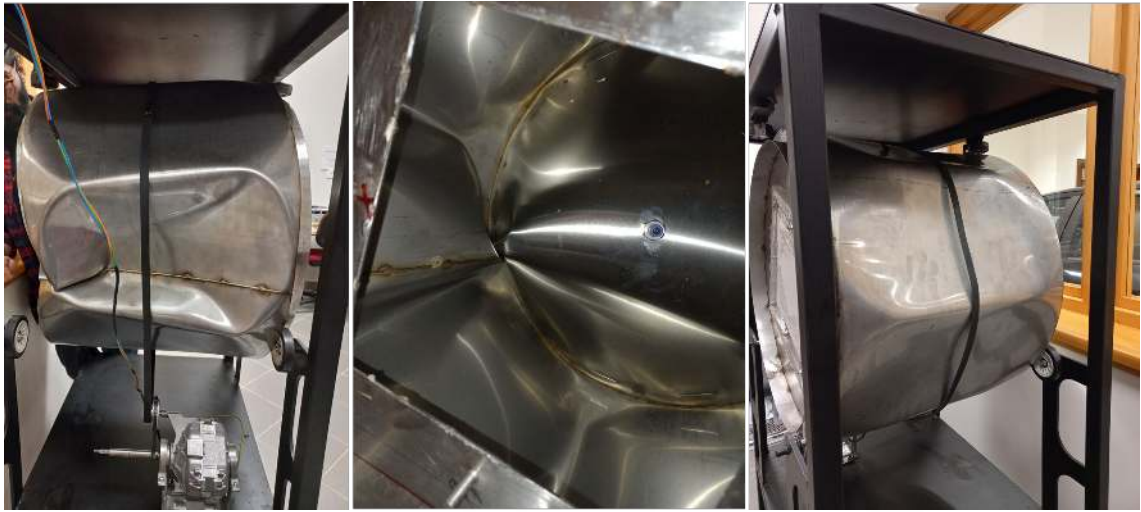
Figure 2.34: Buckled drum pictures.
