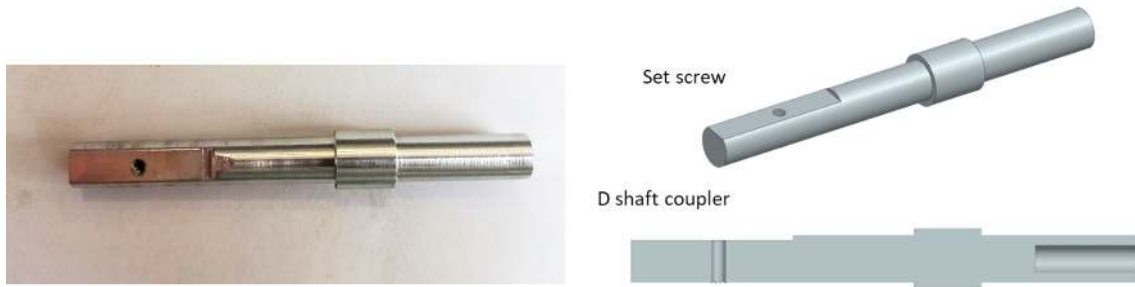
Figure 2.15: Modeled and manufactured shaft
