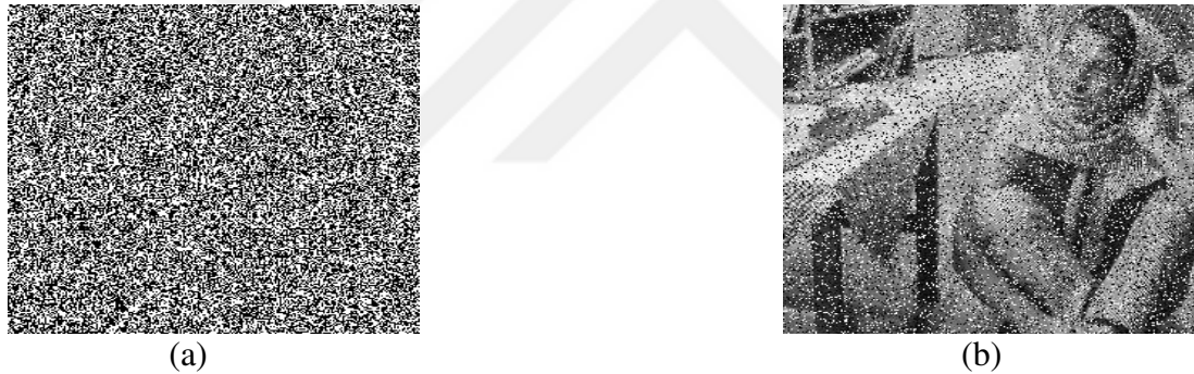
Figure 4. 6 Noise robustness plots: (a) ciphertext image polluted with noise; (b) reconstructed image.
