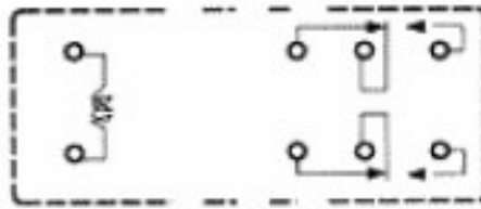
Figure 3.9. YL-221 Power Relay Contact Arrangement (Anonymous, 2006b)
