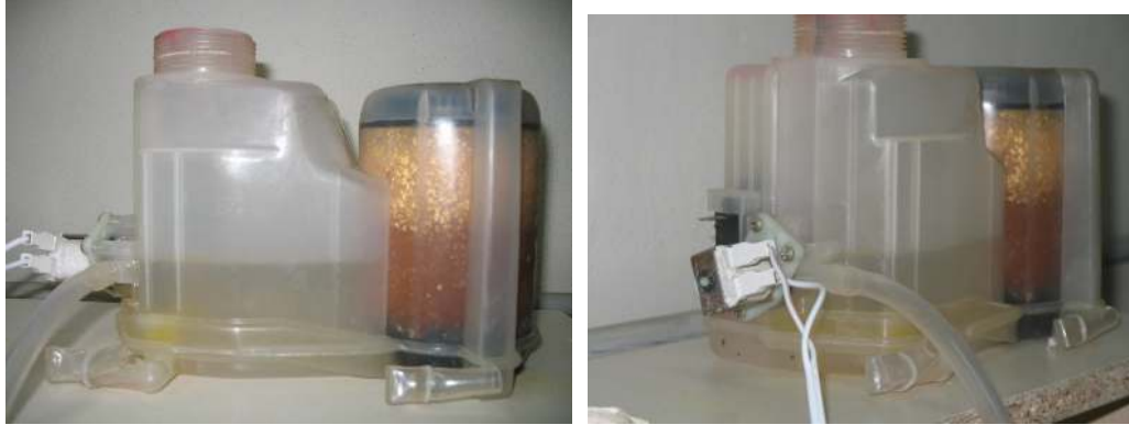
Figure 3.20. Some Photos of the Dosage Pump
