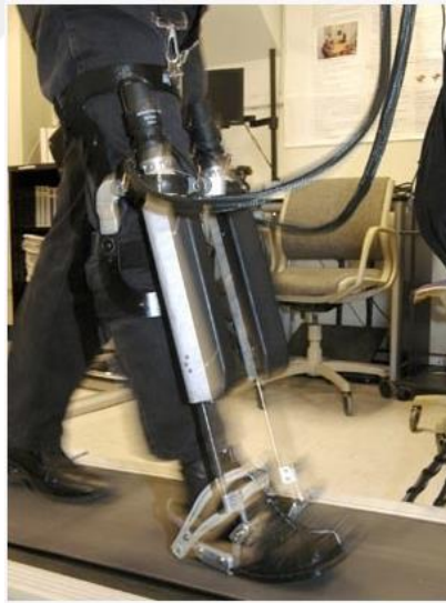
Figure 2-6. The Anklebot active orthoses robotic device (Roy et al., 2009).
