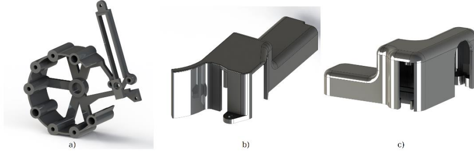
Figure 3-14. The main parts of the backpack mechanism that will be printed. a) Sagittal motor connection, b) Sagittal wire covering, c) Frontal wire covering.
