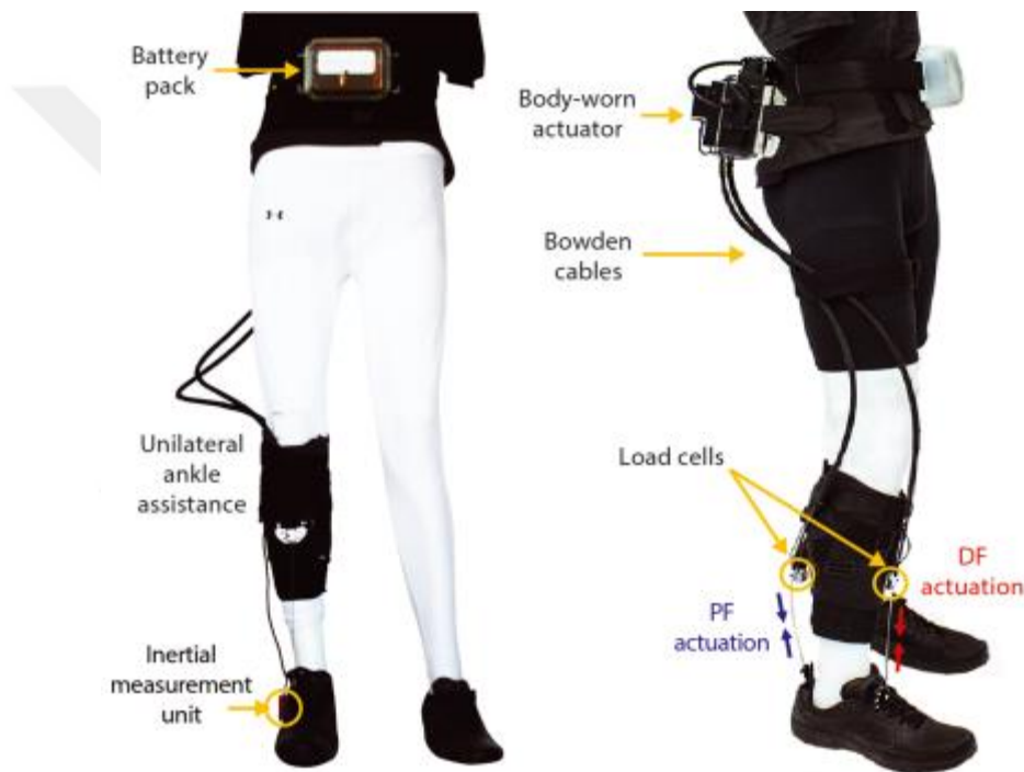
Figure 2-10. A soft wearable robot design with cable-based mechanical power transmission. Plantarflexion (PF) actuation and dorsiflexion (DF) actuation is shown. (Awad et al., 2015).
