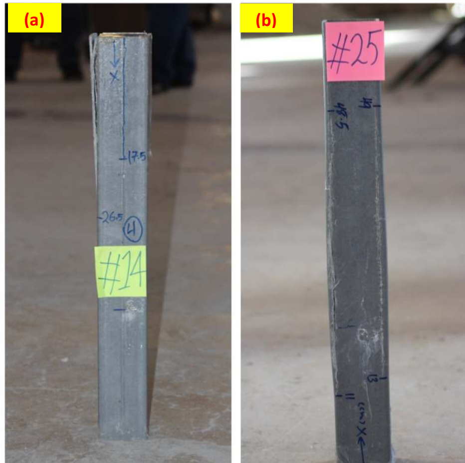
Figure 5.10 (a)-Vertical crack in filled specimen, (b)-Vertical crack in empty specimen
