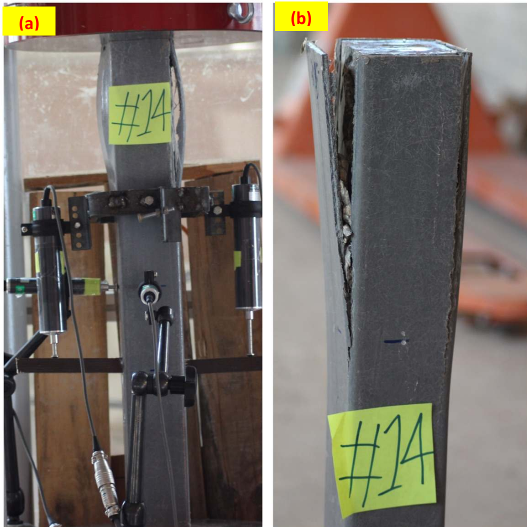
Figure 5.9 (a)-weak interface bond, (b): Tube and concrete separation
