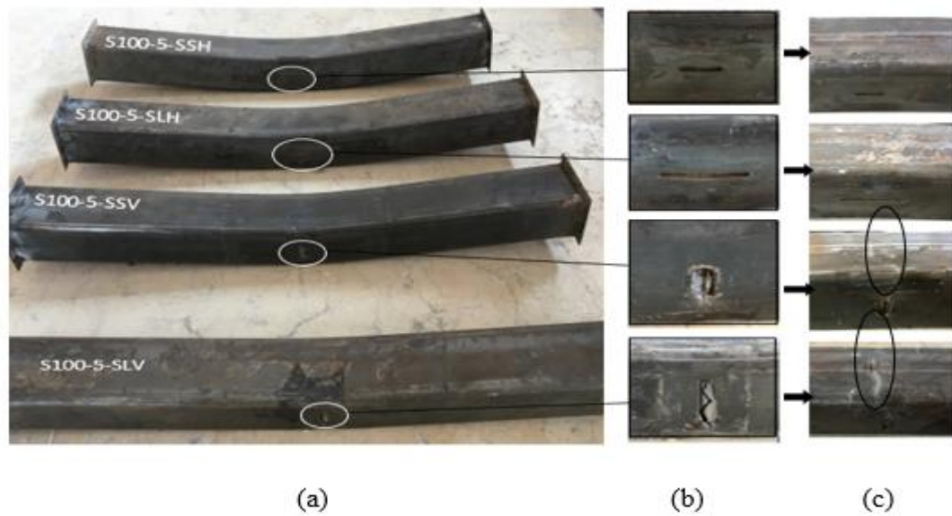
Figure 4.3 Failure modes (a), deformation of the notch (b) and rupture the specimens for GR3(c).
