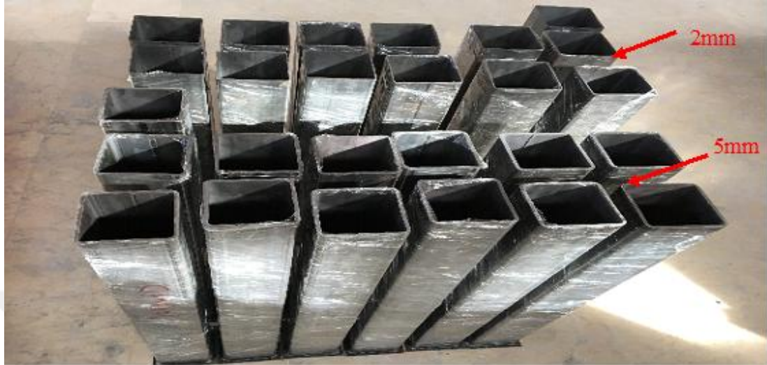
Figure 3.5 Thirteen specimens from each cross section with thickness differences.
