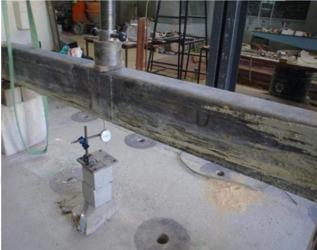
Figure 2.3 Flexural testing of specimens (Ammari et al., 2013).
