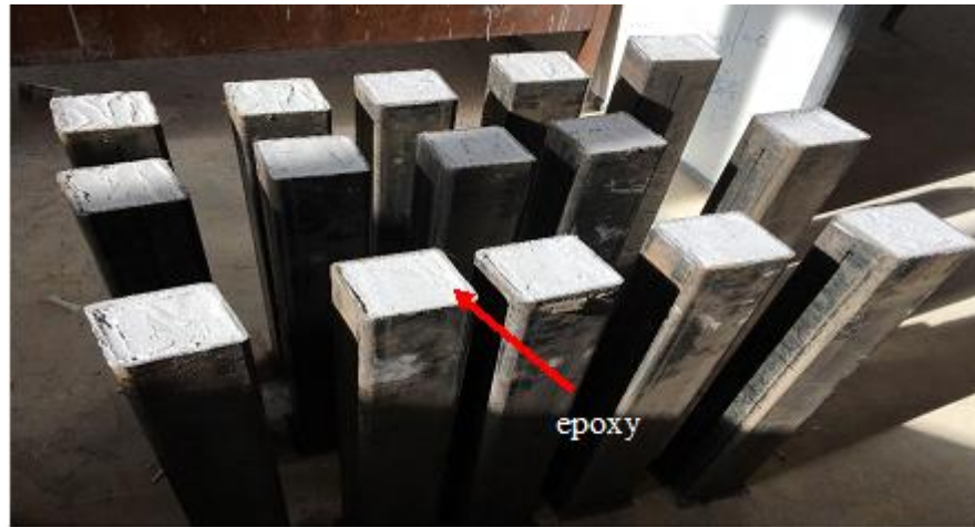
Figure 3.7 The gap filled with epoxy.
