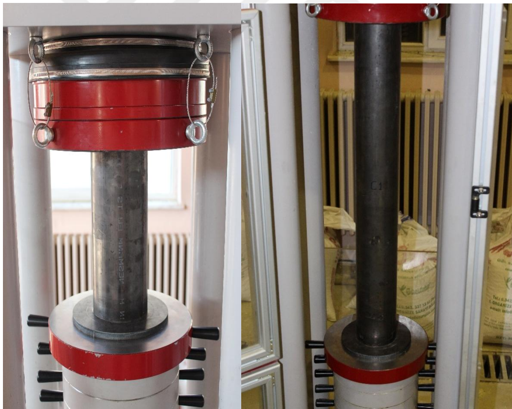
Figure 5.2 CFST column specimen testing setup
