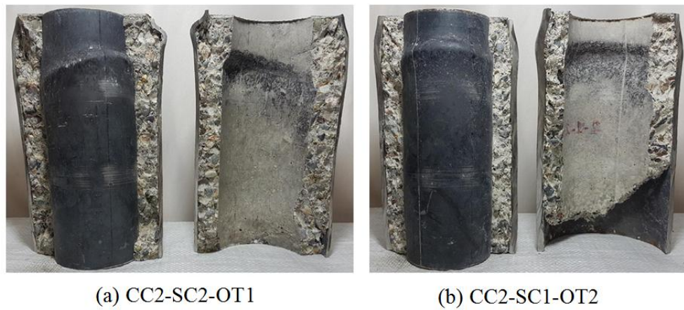
Figure 8.18 Failure modes of columns CC2-SC2-OT1 and CC2-SC1-OT2
