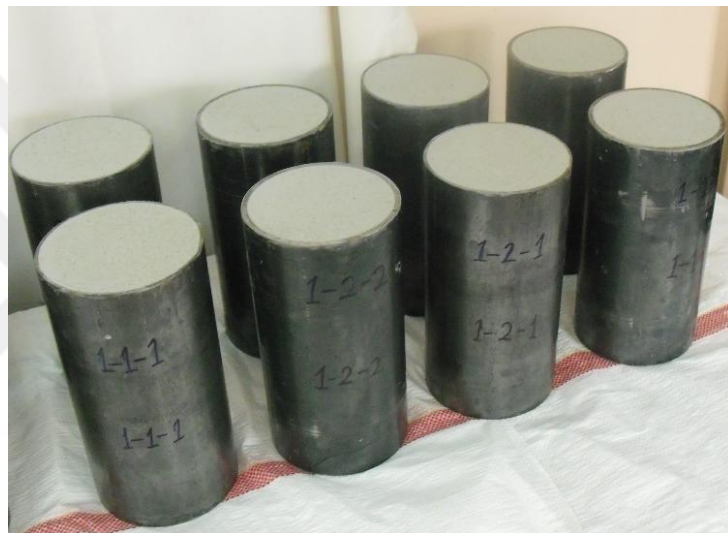
Figure 8.7 Intact CFDCST columns specimens before testing
