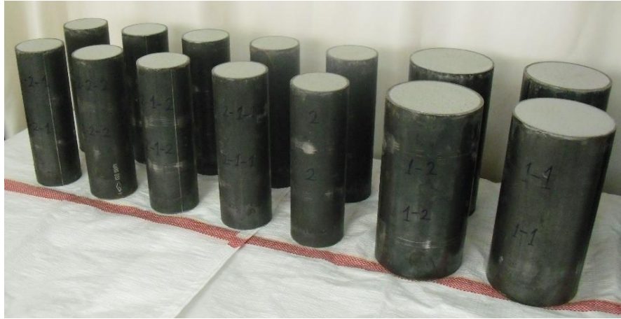
Figure 8.6 Single CFST columns before testing
