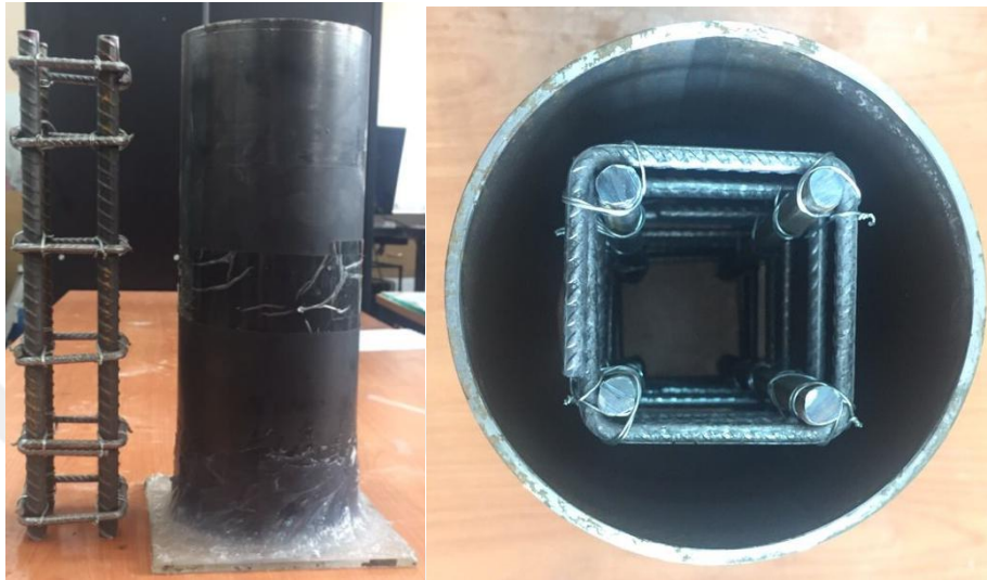
Figure 7.6 Reinforcement and steel tube for a specimen with L/D = 2.62
