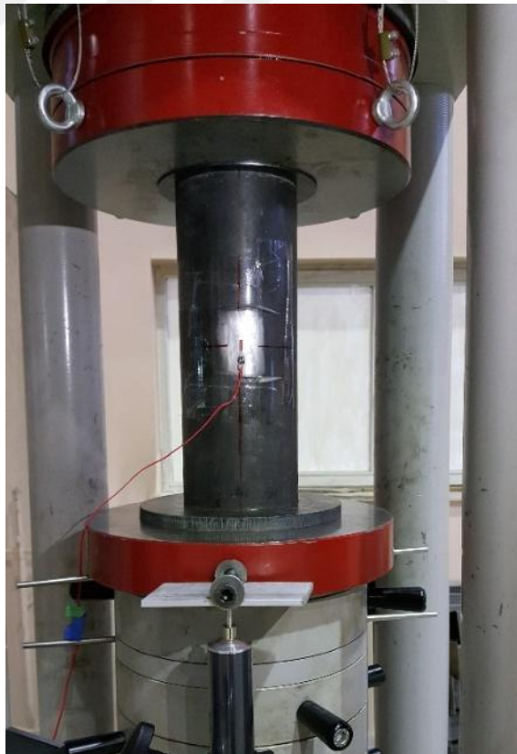
Figure 7.8 RLWCFST specimen testing
