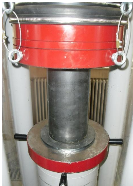
Figure 8.8 Column specimen testing
