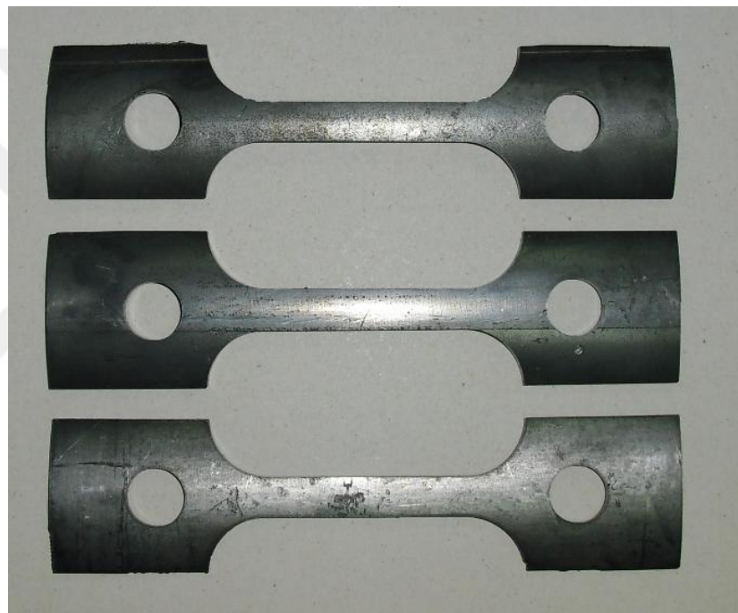
Figure 4.4 Representative tensile coupon specimens
