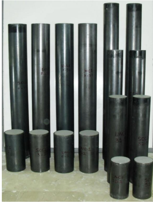
Figure 6.4 CFST column specimens before testing
