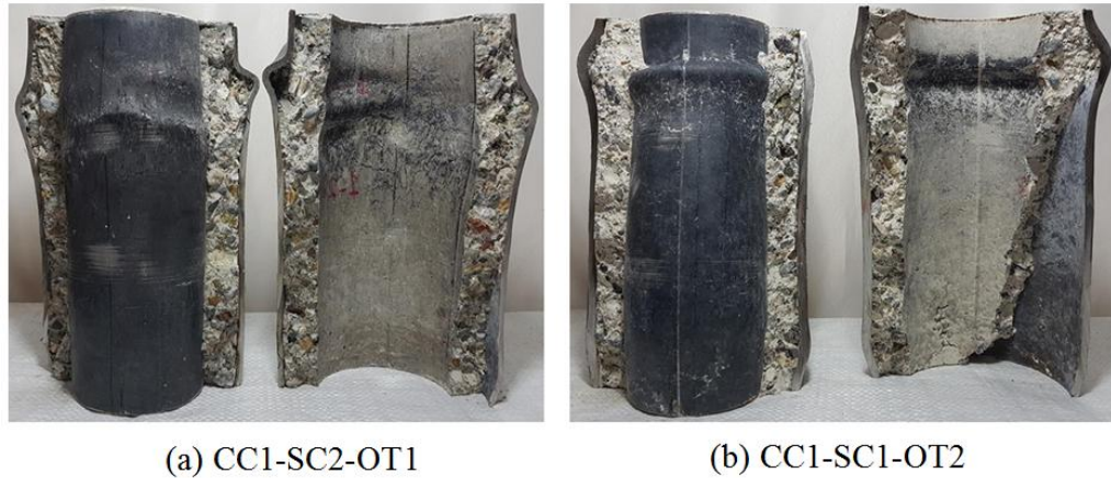
Figure 8.13 Failure modes of columns CC1-SC2-OT1 and CC1-SC1-OT2
