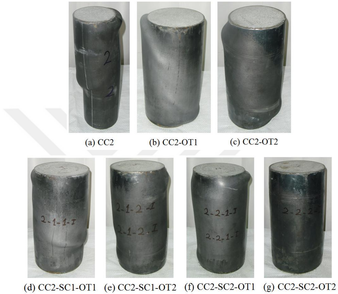
Figure 8.17 Failure modes of columns with HS core concrete
