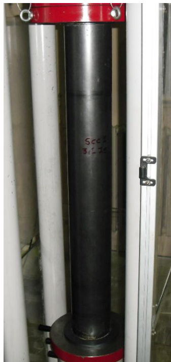
Figure 6.5 CFST column specimen test
