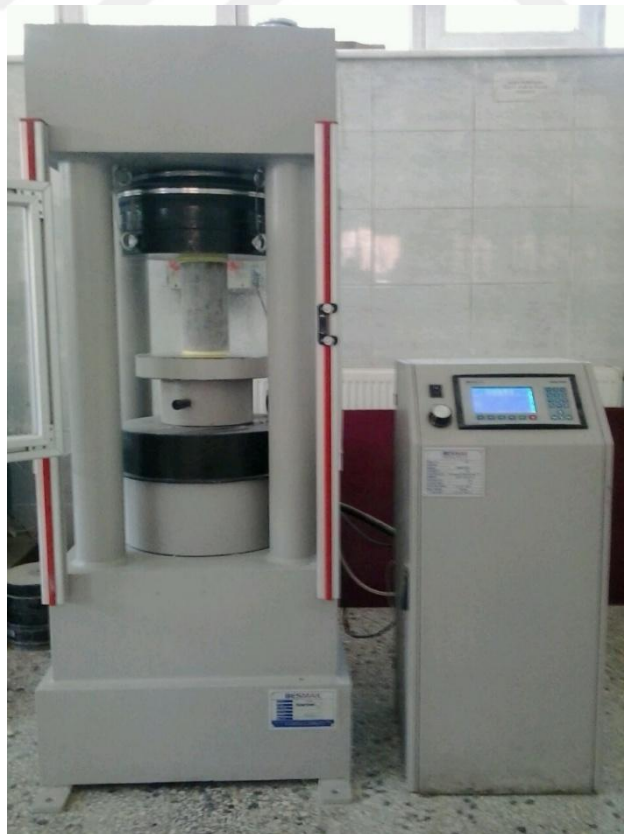
Figure 4.9 Testing machine used for concrete specimens
