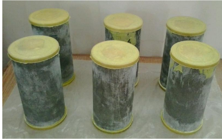
Figure 4.10 Samples of concrete specimens before crushing
