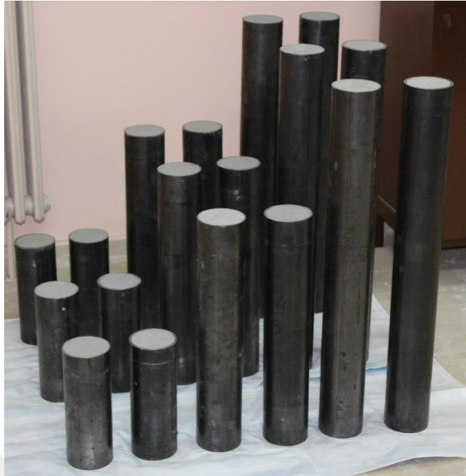
Figure 5.1 CFST column specimens before testing
