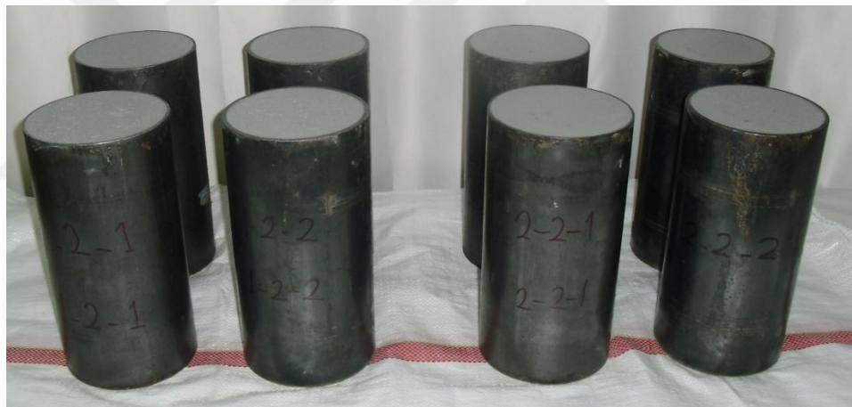
Figure 8.20 Composite columns of repair configuration before testing
