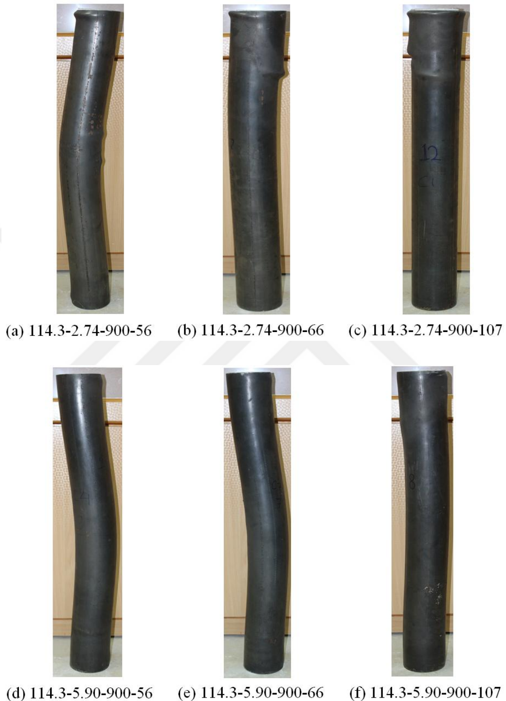
Figure 5.8 Failure modes of long columns
