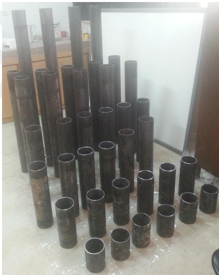
Figure 4.2 Steel tube specimens before pouring concrete
