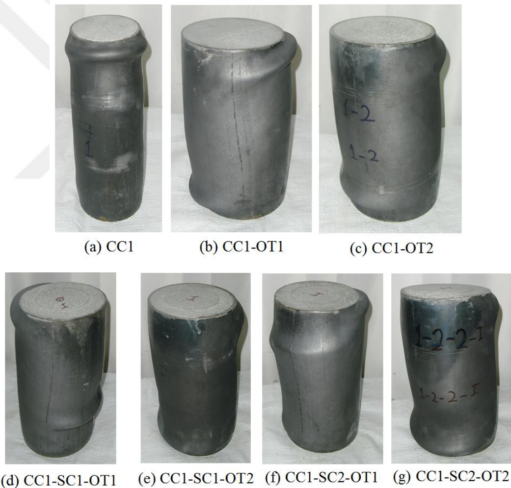
Figure 8.12 Failure modes of columns with NS core concrete
