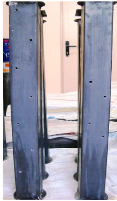
(b) Drilled SCCFST beams
