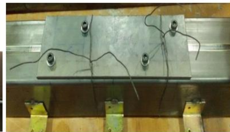
(d) Application of epoxy and installation of bolts through holes
