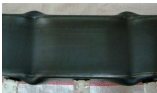
(b) Inward local buckling of beam H120-120-2.80
