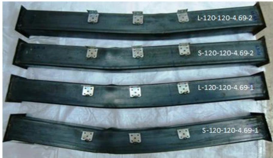
(c) 120×120×4.69 mm CFST beams
