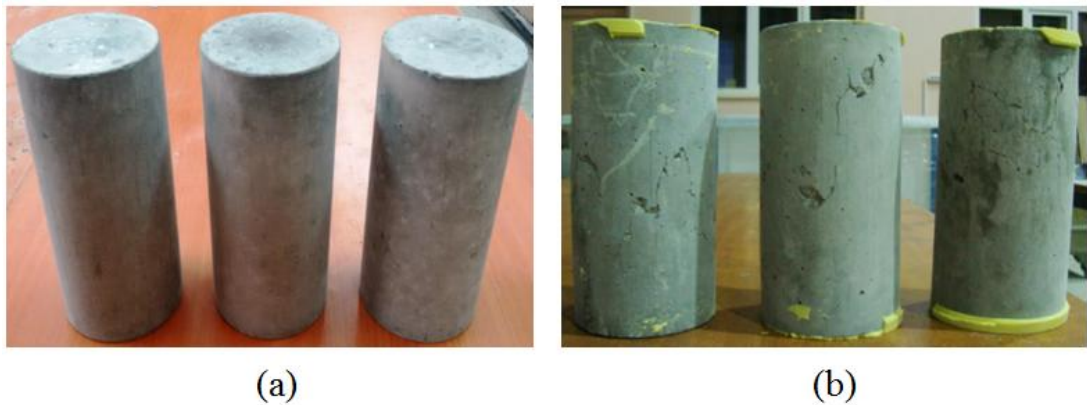
Figure 5.1 Concrete cylinders (a) before testing, (b) after testing
