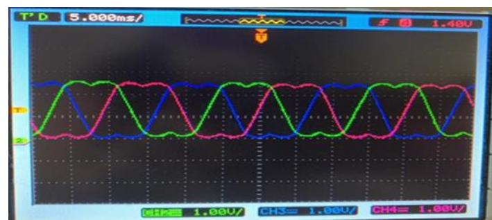
Figure 6.28. The result of harmonics before comparing with triangular wave (practical)
