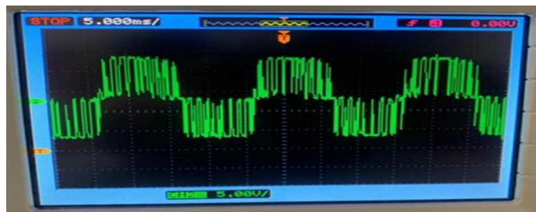
Figure 6.34. Line to line voltage when 10 volt is give to inverter
