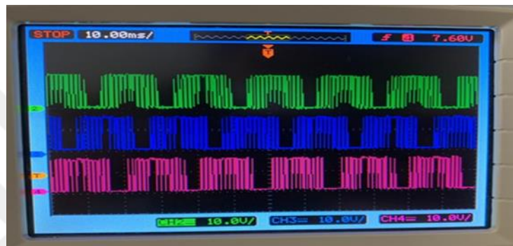
Figure 6.30. SVPWML1, SVPWML2 and SVPWML3(practical)
