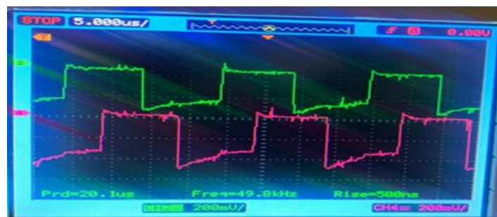
Figure 6.37. The pulses of the encoder in practical
