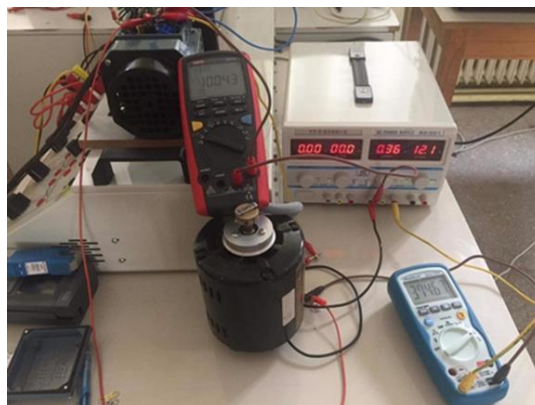
Figure 5.1. DC Test of 0.25 kW three-phase IM
