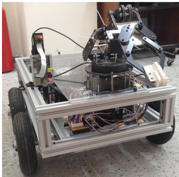
Figure 3.32 The mobile manipulator after mounting
