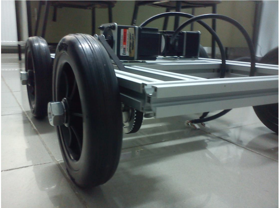
Figure 3.26 Mobile platform after mounting of wheels and motors
