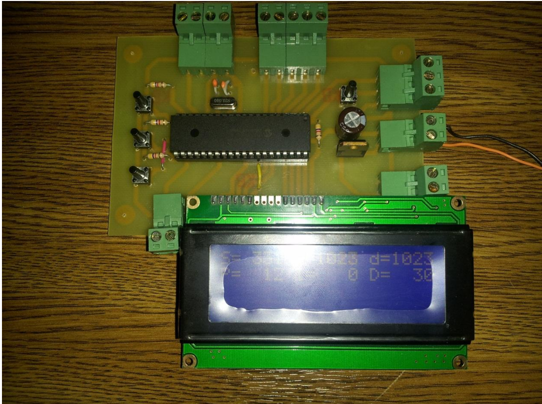
Figure 4. 8. A photo of MCU circuit with LCD
