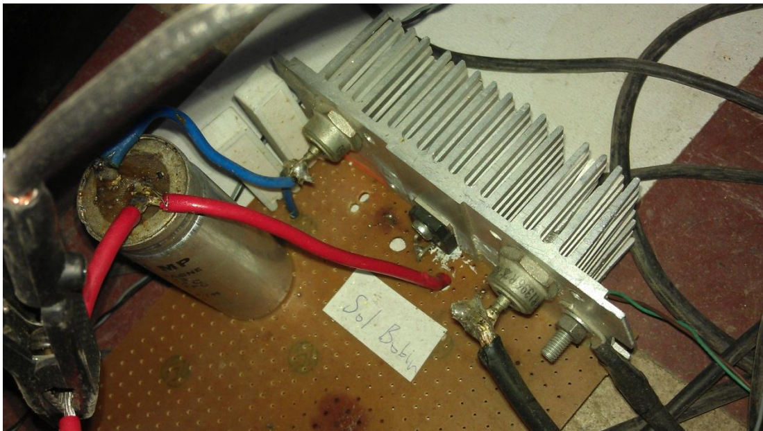
Figure 4. 15. Snubber circuit with Power Mosfet
