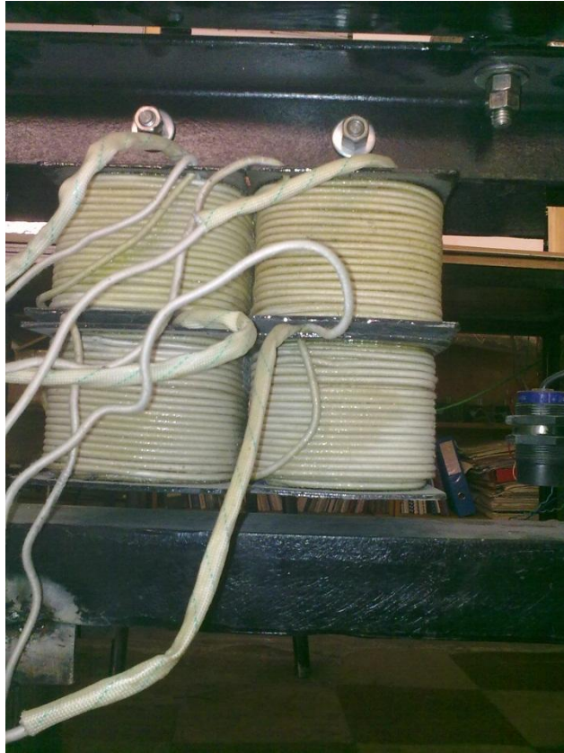
Figure 5. 15. SAEMSS using u-type electromagnet
