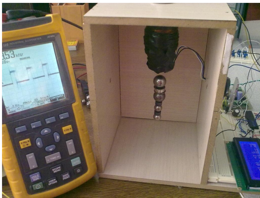
Figure 5. 14. SAEMSS using solenoid type electromagnet with two different weights
