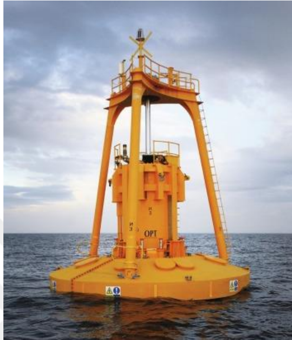
Figure 2.21. The OPT WEC (Neill and Hashemi, 2018)
