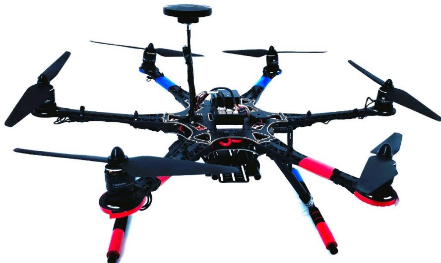
Figure 3.3 Assembling of hexacopter frame and components (Manjarrez et al. 2023)
