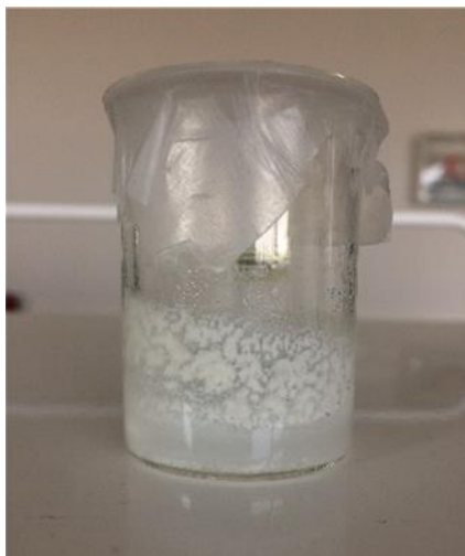
Figure 4.4. Exp 3, Genipin crosslinked HSA nanoparticles 25°C for 24 hours
