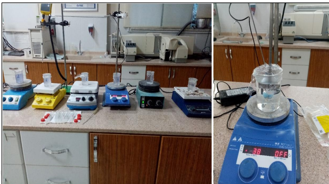
Figure 11.7 Dialysis membranes positioned in beakers filled with 250 mL of simulated gastric fluid and kept on a magnetic stirrer at 37°C.
