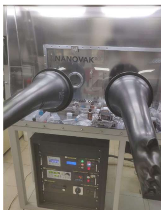
Figure 4.4 Nanovak thermal evaporator located inside the glovebox.
