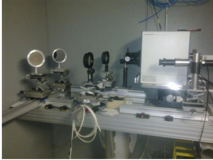
Figure 4.4: Alignment of the mirrors and lenses with a laser.
