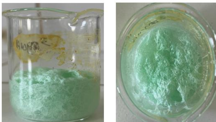
Figure 4.2 The dried gel of \text{Mg}_{0.003}/\text{Cu}_{0.0001}/\text{Al}_{0.001} obtained after heated at 105^{\circ}\text{C} for 24H
