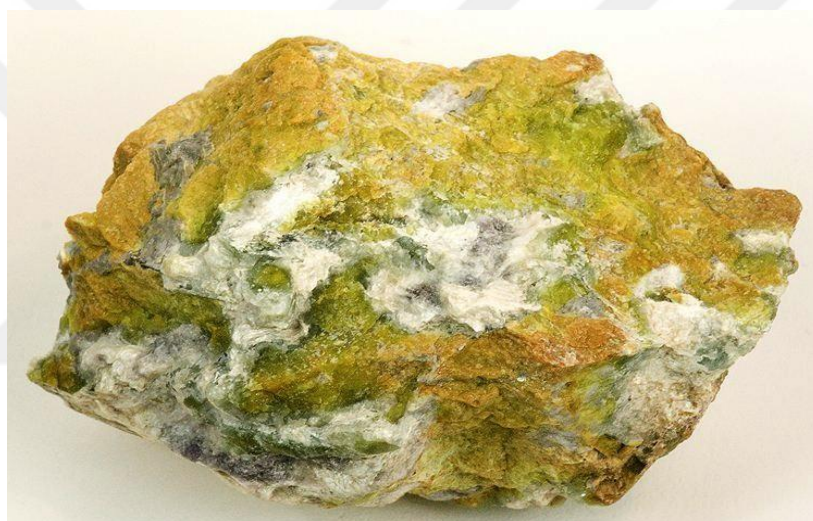
Figure 1.1 Hydrotalcites \text{Mg}_6\text{Al}_2(\text{OH})_{16}(\text{CO}_3) \cdot 4\text{H}_2\text{O} .
