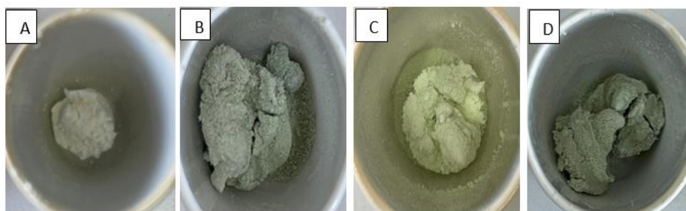
Figure 4.5 A) MgAl, B) MgCuAl, C) MgNiAl, D) MgCuNiAl obtained after heated 650^{\circ}\text{C} mix metal oxides (MMO).
