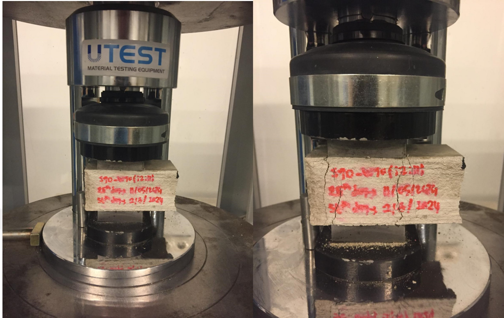
Figure A.2: Compressive strength test apparatus with test sample
