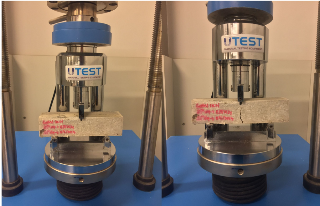
Figure A.1: Flexural strength test apparatus with test sample
