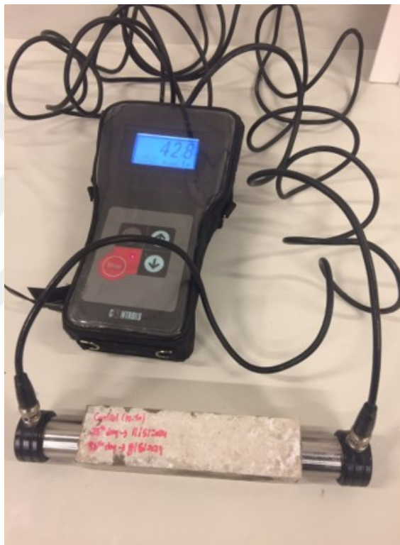
Figure A.4: Application of UPV test in test sample
