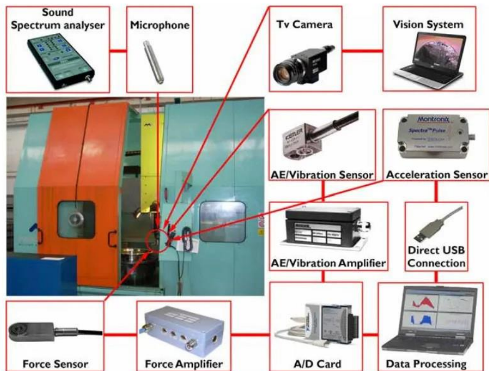
Figure 49: Example of a multi-sensor CNC process monitoring acquisition setup
