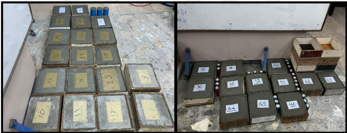
Figure 2.6. Freshly cast specimens kept in their molds for 24 hours prior to demolding
