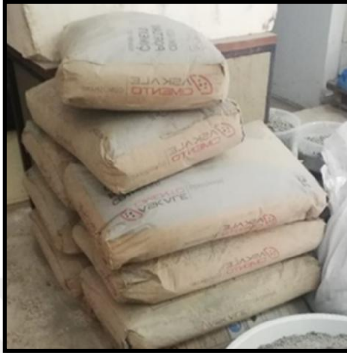
Figure 2.2. Portland cement type CEM I 42.5 R manufactured by the Akçakale Manufacturing Group, Trabzon, used as the binder in sample preparation
