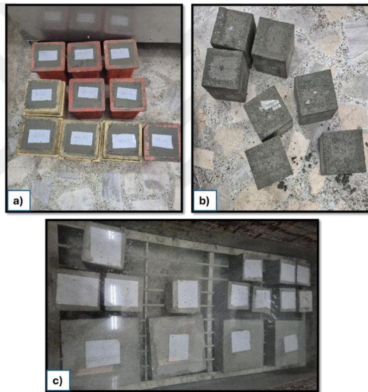
Figure 2.15. Casting, demolding, and curing of 100 \times 100 \times 100 mm concrete cubes: (a) placement and compaction; (b) demolding after initial set; (c) water curing at 18 \pm 2 °C for 7 days.
