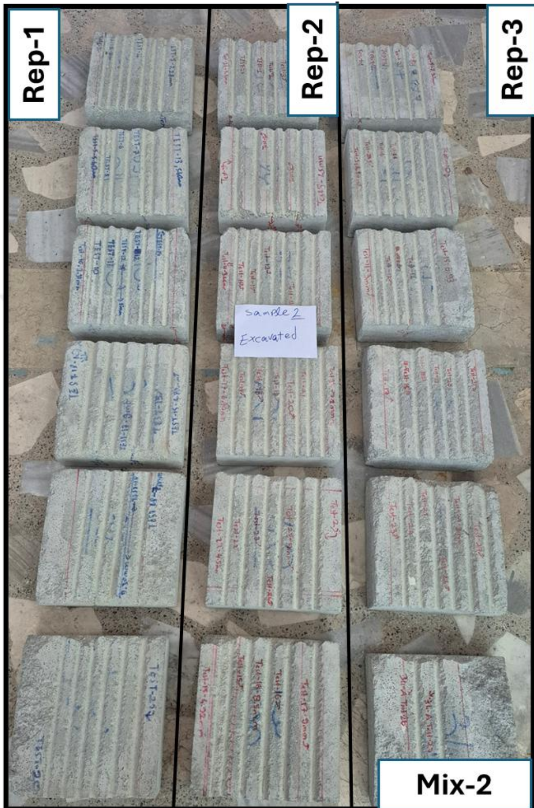
Figure 2.26. Mix-2 complete specimen set after three rotary unrelieved cutting repeats
