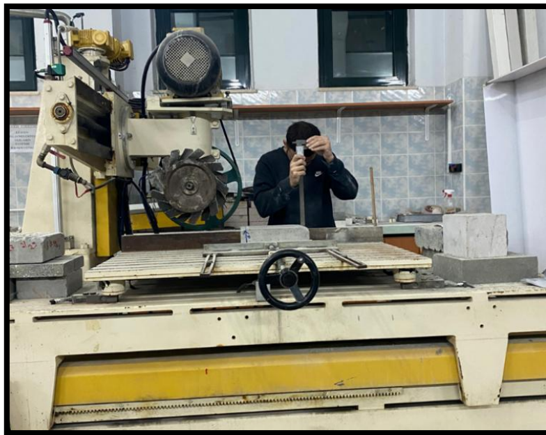
Figure 2.23. Post-cut verification of the real depth of cut using a digital vernier caliper on grooves
