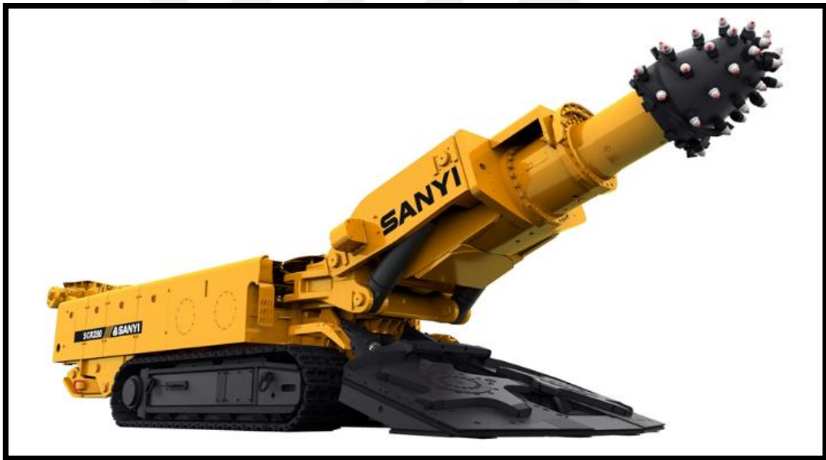
Figure 1.3. Axial roadheader- SANY SCR280 High-Gradient axial roadheader (SANY)
