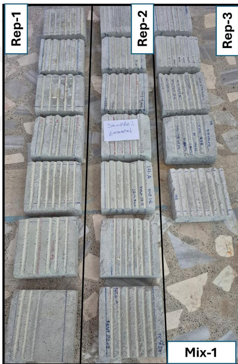
Figure 2.25. Mix-1 complete specimen set after three rotary unrelieved cutting repeats
