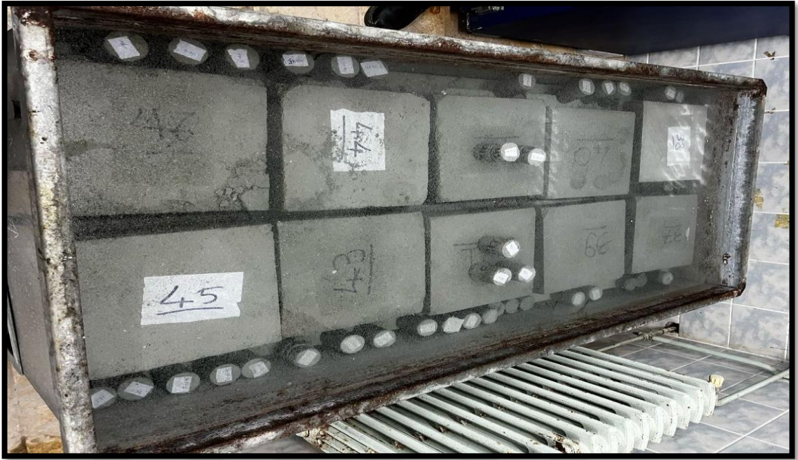
Figure 2.7. Concrete specimens submerged in a water tank during the curing stage
