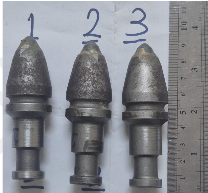
Figure 3.39. Visual condition of Picks 1–3 after cutting tests.
