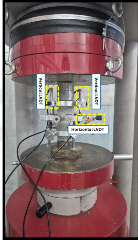
Figure 2.19. LVDT layout for modulus test; two vertical and one horizontal on the specimen, mounted over the gauge length per ISRM
