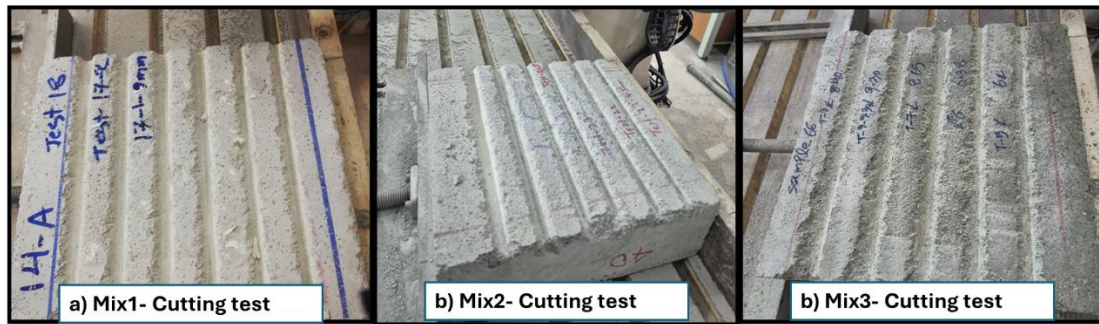
Figure 2.24. Representative specimens after rotary unrelieved cutting: (a) Mix 1, (b) Mix 2, (c) Mix 3
