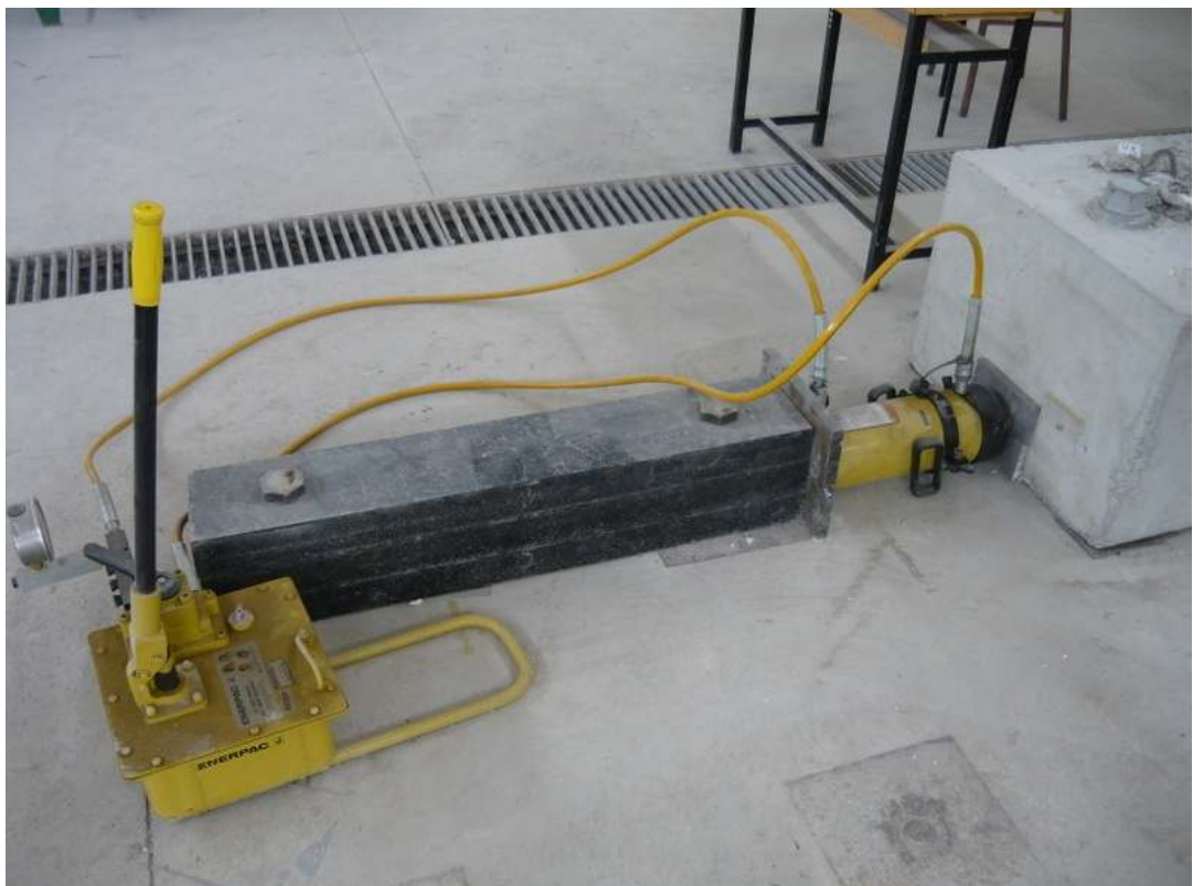
Figure 3.25 Hydraulic rams which constrain foundation
