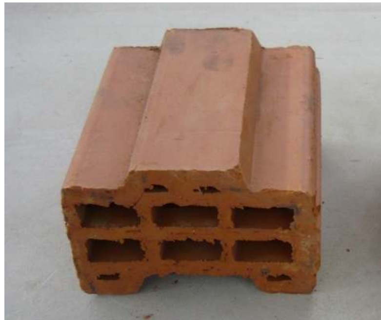
Figure 3.6 Locked brick with a scale of \frac{1}{2}
