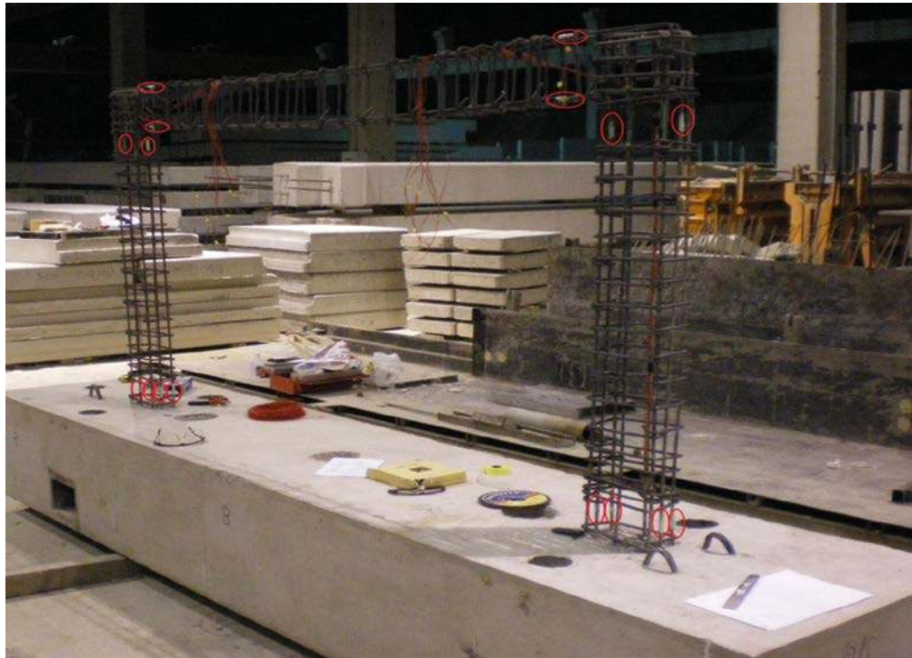
Figure 3.14 Reinforcements were applied strain gauge
