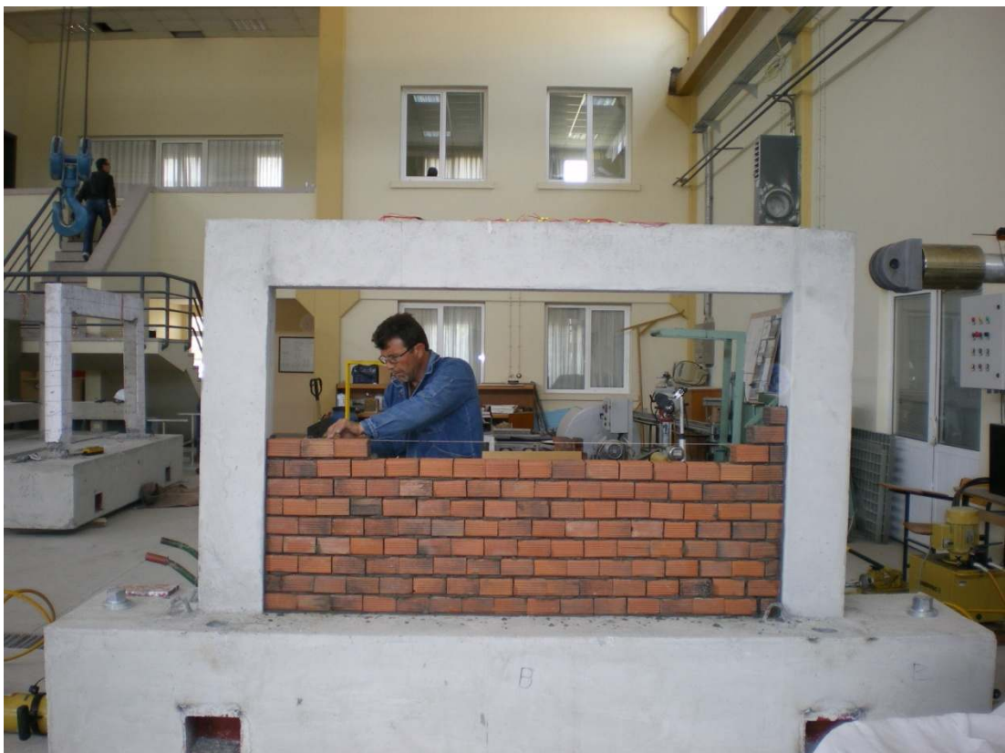
Figure 3.11 Standard brick construction
