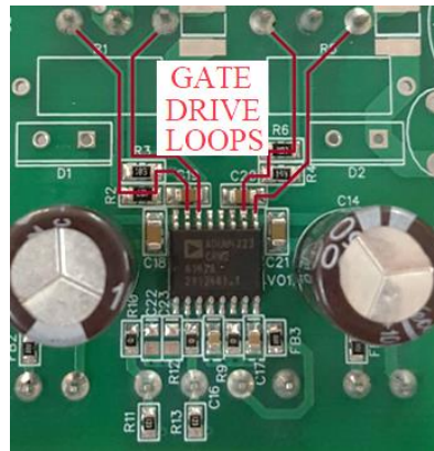
Figure 3.25 Isolated gate driver circuit and corresponding current loops (Personal archive, 2018)
