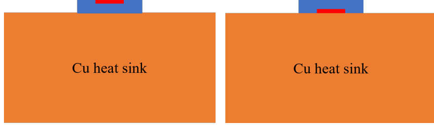
Figure 1.8: Schematic of (a) epi-up & (b) epi-down mounting.
