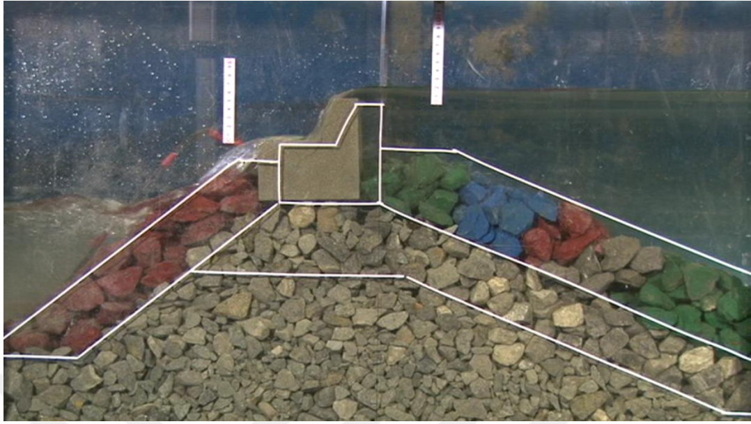
Figure 3.4. Sliding of the Crown-Wall in the Tsunami Overflow Experiment on the Original Cross-Section ( h=1.9 cm)
