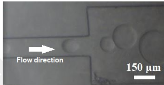
Figure 2.23: Optical Microscope image showing droplet merging at the entrance of the wider channel because of absence of any surfactant.
