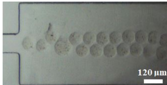
Figure 3.5: Optical microscope image showing the magnetic nanoparticles spread uniformly in the droplets.
