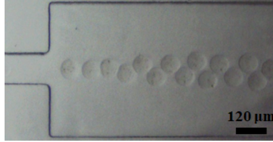
Figure 3.6: Optical microscope image showing the magnetic nanoparticles spread uniformly in the droplets.
