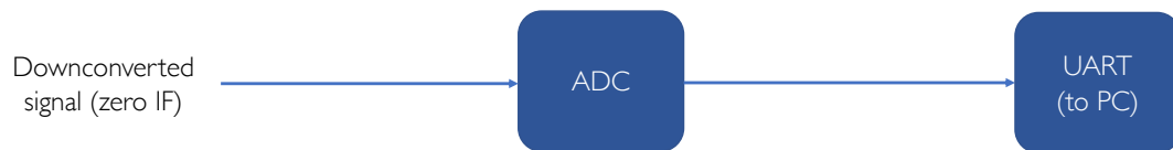
Figure 3.14: Illustration for the initial plan. Oscillator's output will be downconverted, sampled, and transmitted to PC.
