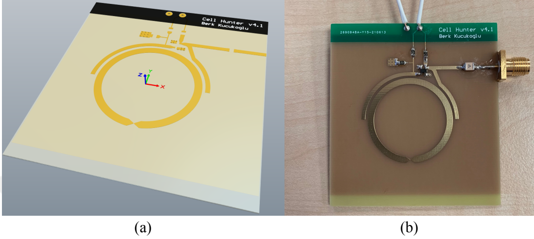
Figure 3.7: (a) Oscillator layout designed in Altium Designer, and (b) manufactured design.
