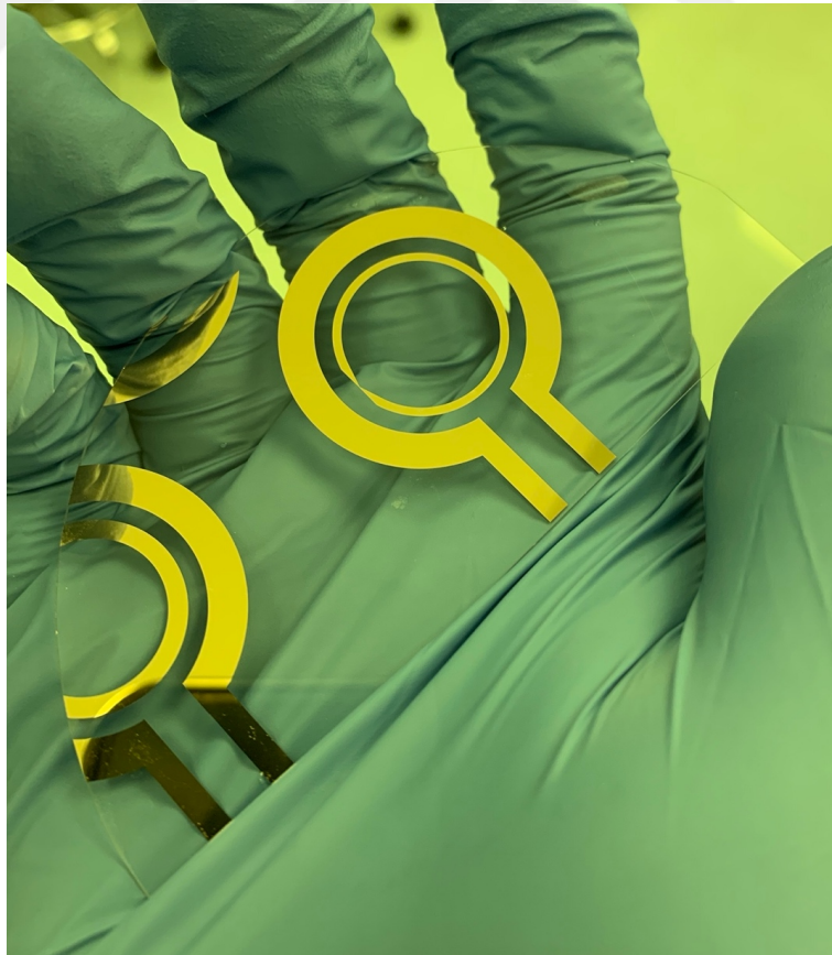
Figure 2.13: Photo of the final CSRR device on diced quartz wafer.
