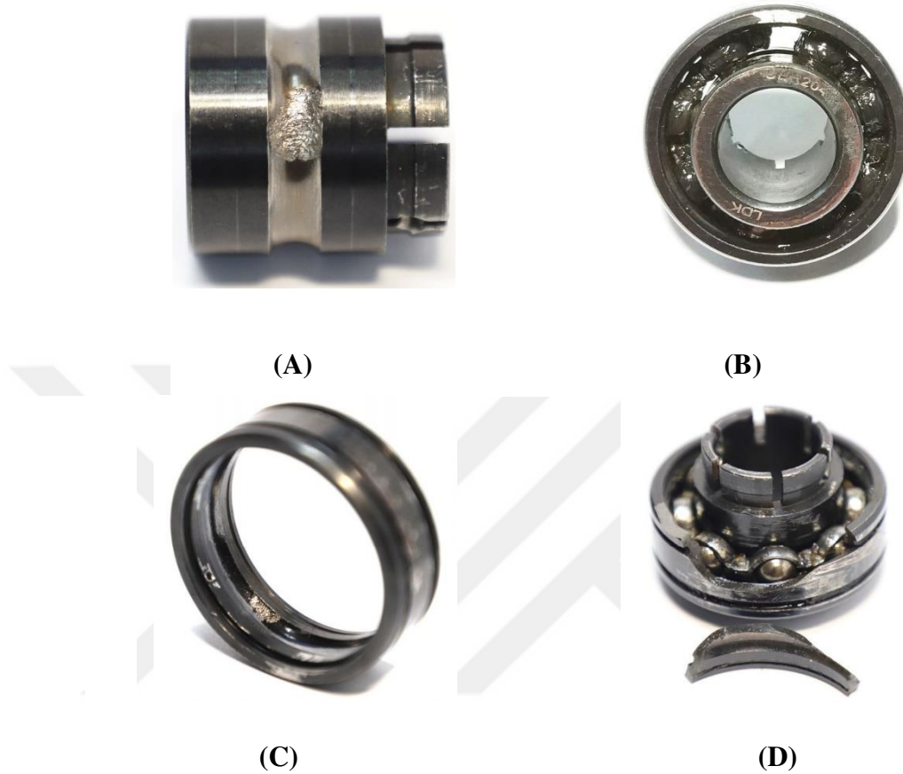
Image 2.8. Demonstrated Diverse Types of Damages Inflicted on the Bearings During the Experimental Study (A) Inner Race Damage (B) Cage Damage (C) Outer Race Damage (D) Outer Race Fracture
