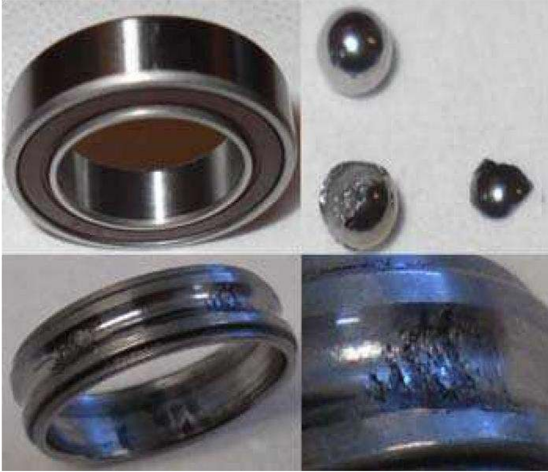
Image 2.5. Showing a Normal and Damaged Bearing Before and After Operations on PRONOSTIA
