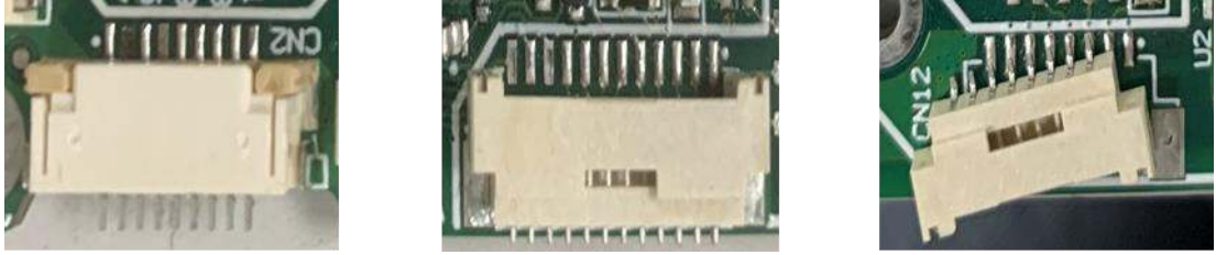
Figure 2.5 Examples of Connector Defect.
