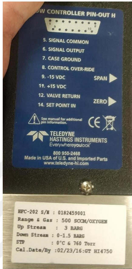
Scheme 2-7. An MFC casing indicating calibration conditions and MFC specific parameters.
