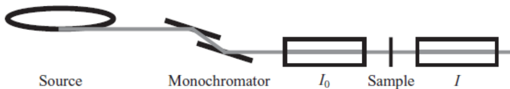
Appendix C5. The schematic illustration of transmission-based EXAFS experiments [290]. Copyright (2020) Wiley.
