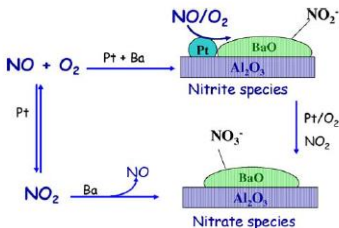
Scheme 1-1. Representative scheme for NO x removal on Pt/BaO/Al 2 O 3 [16]. Copyright (2020) Elsevier.
