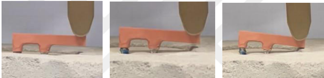
Fig 4.5. – 4.7. (Left) PE2101 framework reciprocating 175 N, load arm extension 2,51 mm, not decemented yet, (Middle) PE2101 framework decemented, reciprocating 150 N, (Right) PE2101 framework dislocated after reciprocating 200 N
