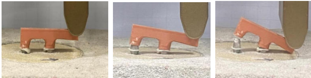
Figure 4.1. – 4.3. (Left) PE1401 Framework reciprocating 330 N, load arm extension 1,2 mm, not decemented yet, (Middle) PE1401 Framework decemented, reciprocating 110 N, (Right) PE1401 Framework dislocated after reciprocating 200 N
