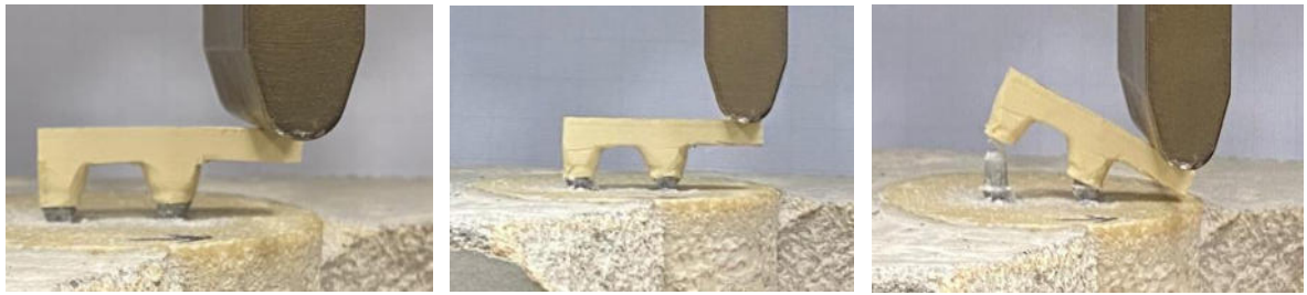
Figure 4.15. – 4.17. (Left) BH1401 framework reciprocating 210 N, load arm extension 1,22 mm, not de-cemented yet, (Middle) BH1401 framework de-cemented, reciprocating 200 N, (Right) BH1401 framework dislocated after reciprocating 292,5 N
