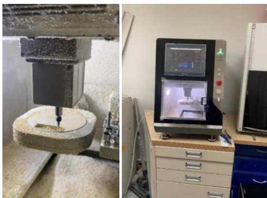
Figure 3.13. (Left) PEEK blank is getting milled
