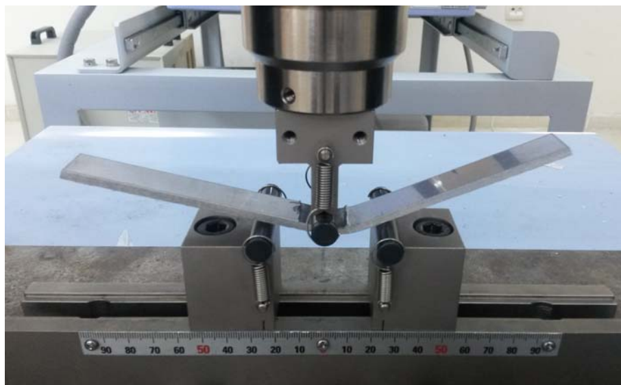
Figure 6.7 Bending test in progress (Personal archive, 2017)
