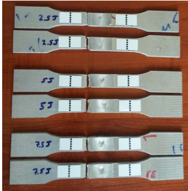
Figure 7.18 Fracture locations of the impact-tested specimens after tensile tests (Oztoprak, Yeni & Kiral, 2018b)
