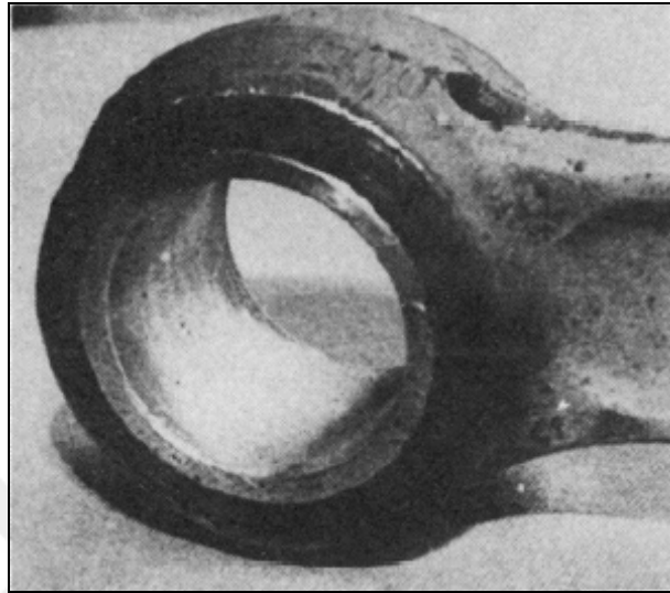
Figure 2.9 A bearing manufactured from cast Al/graphite composite (Rohatgi, 1991)
