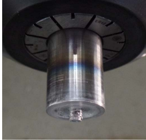
Figure 5.4 Fabricated welding tool used for FSW process (Personal archive, 2016)
