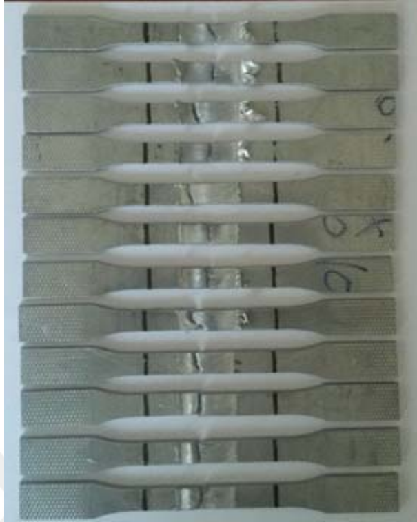
Figure 8.13 Failure locations of the FSWed joints (Oztoprak, Yeni & Kiral, 2018c)
