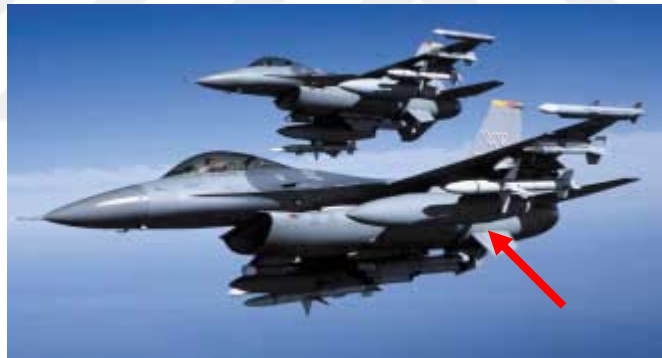
Figure 2.7 The F-16 jet fighter contains ventral fins and fuel access door covers made from the AMC. The composite ventral fin is displayed by the red arrow (Hunt & Herling, 2004)
