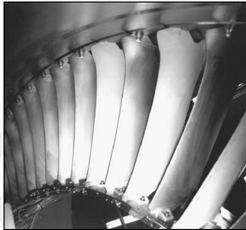
Figure 2.8 AMC application in guide vane assembly of the Trent engine (Hooker and Doorbar, 2004)
