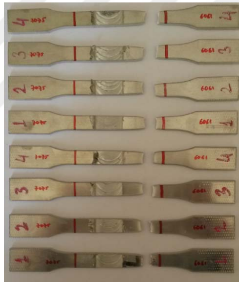
Figure 5.16 Failure positions of the tensile test specimens (Personal archive, 2016)
