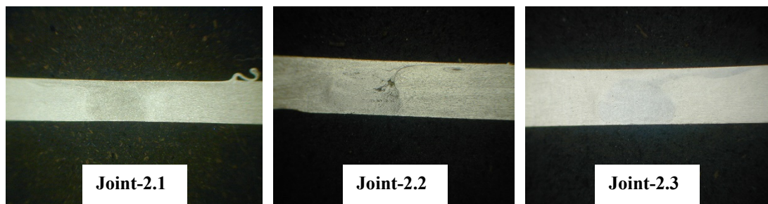
Figure 5.5 Macrostructures of the friction stir welded AA6061-O (Personal archive, 2016)
