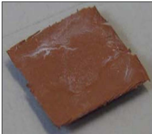
Figure 2.12 Thin foil made from copper-CNT composite (Aryasomayajula & Wolter, 2013)
