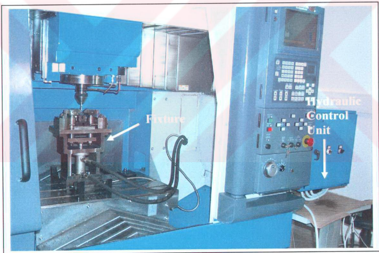
Figure 6.20: Experimental setup of measuring cutting forces for cylindrical surfaces
