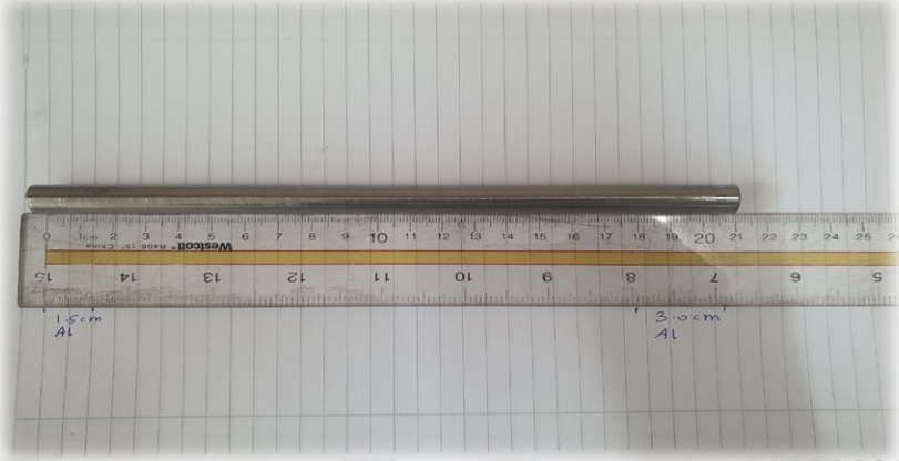
Photo 7.2 Iron sheath with \text{Mg}+2\text{B} powder inside.
