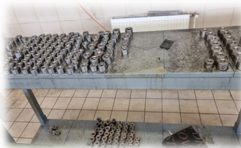
c) Tungsten Carbide Dies (inner diameter from 0.5 mm to 15 mm)
