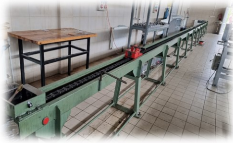
a) Drawing machine (17 meters)
