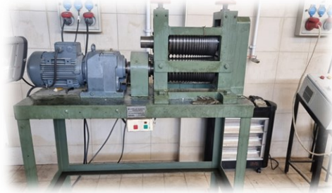
b) Rolling machine (from 1 mm to 15 mm)
