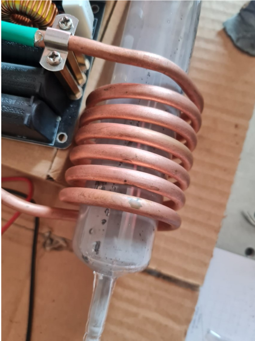
Photo 6.1 Joint of \text{MgB}_2/\text{Fe} wires via our induction heating system.
