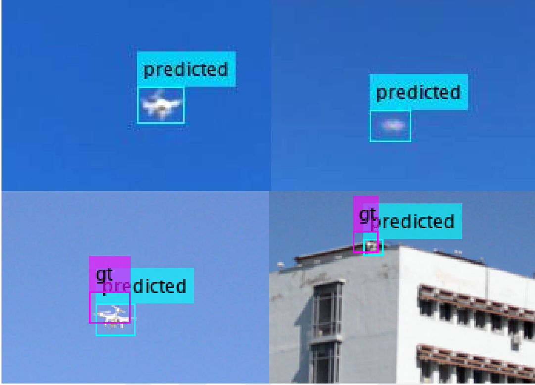
Figure 4.4: At the top, examples of inferred boxes (predicted) which are tabulated as false alarms in Table 4.2 and 4.3; at the bottom examples for the annotations which should be evaluated with \theta_{IoU} = 0.2 instead of \theta_{IoU} = 0.5 due to the shown incorrect original ground-truth (gt). Displayed frames are (a) 8445 of 00001, (b) 7912 of 00002, (c) 3682 of DSC_6299, (d) 1222 of DSC_6304.
