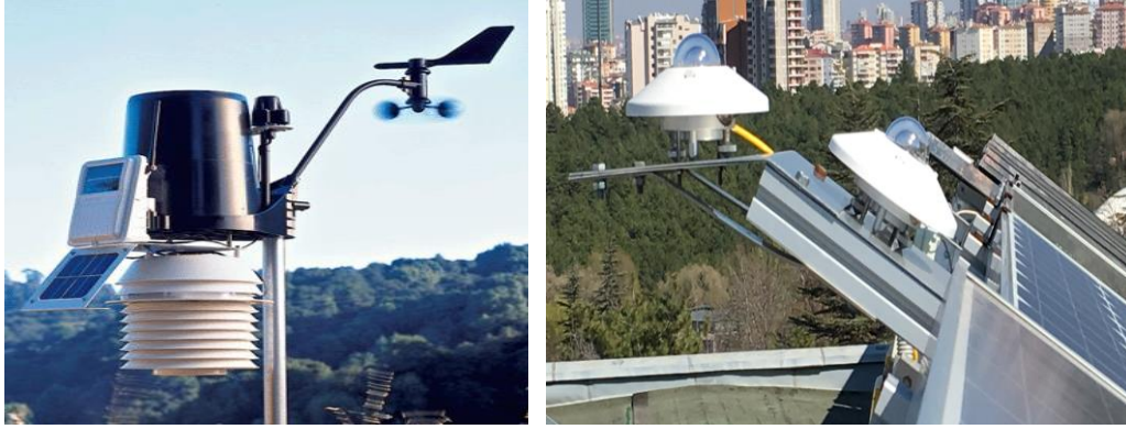
Figure 3.3. Meteorological Station (Davis Vantage Pro2+) and sensors (Kipp&Zonen CMP11)
