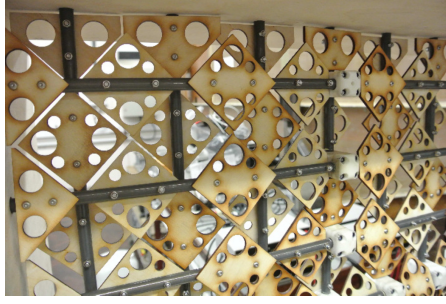
Figure 4.2: Cut-out wings used as active grid in Case 1 [27]
