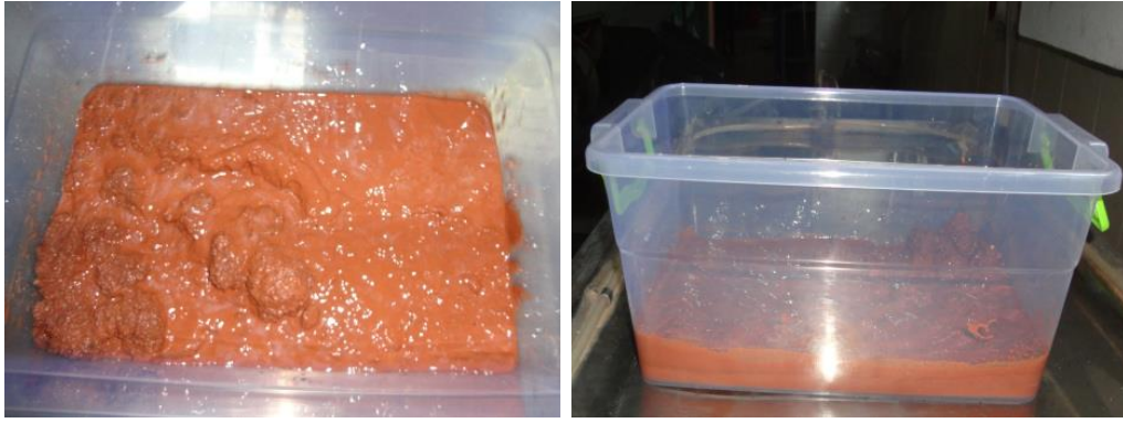
Figure 3.33 : The appearance of bauxite with 10% moisture content exposed to vibration after 3 hour
