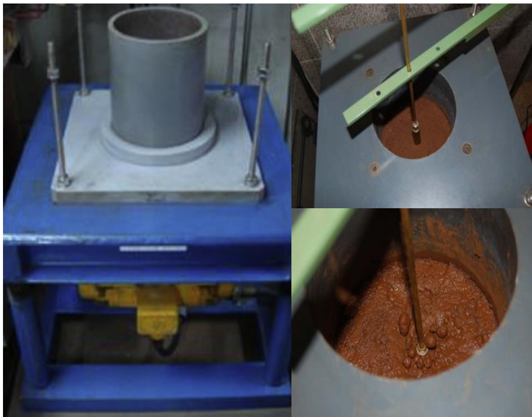
Figure 3.11 Observations on the Penetration Table Test to find TML.
