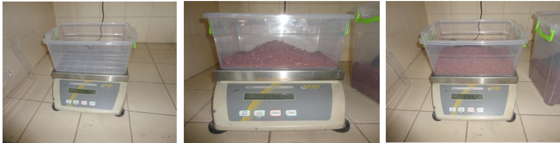
Figure 3.29 : Measuring of the 3000g of bauxite and angle of repose before experiment.
