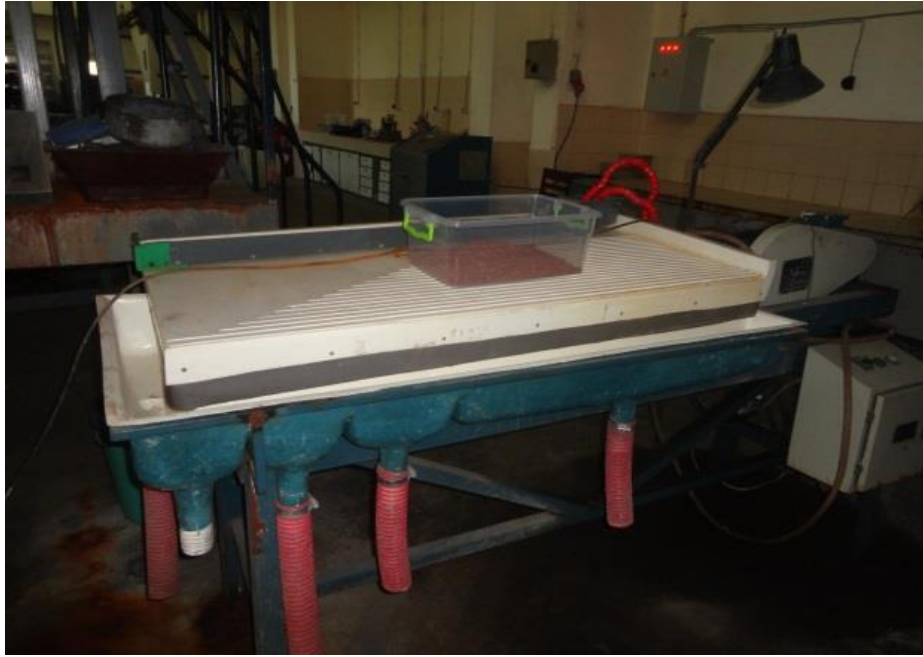
Figure 3.21 : Wilfley shaking table with dried bauxite moisture content less than 1 percent
