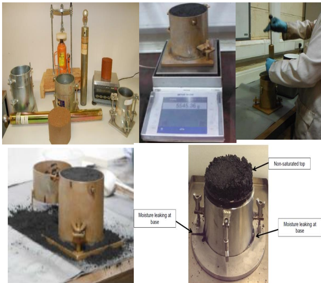
Figure 3.7 : Observations on the Proctor/Fagerberg Table Test to find TML.
