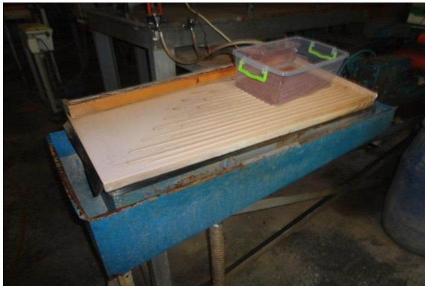
Figure 3.22 : Deister shaking table with bauxite TML 8.9 percent (right).
