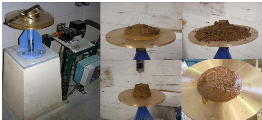
Figure 3.3 : Observations on the The Flow Table Test to find TML.
