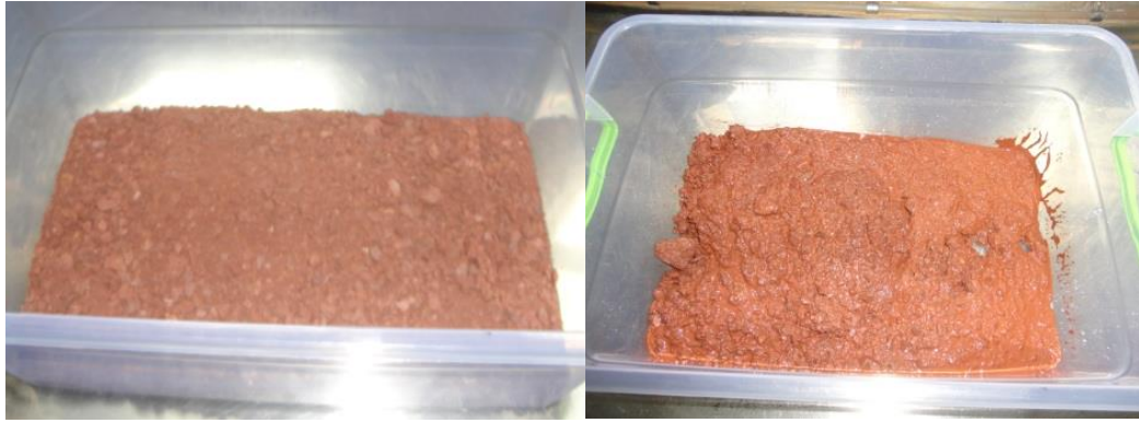
Figure 3.31 : The appearance of bauxite with different moisture content exposed to vibration after 1 hour (left-less1%), (right 10%)
