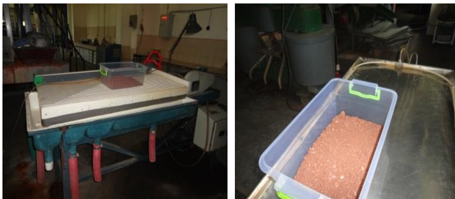
Figure 3.30 : The bauxite less than 1 percent moisture place on wilfley shaking table (left), The bauxite involving 10 percent MC place on deister shaking table (right).
