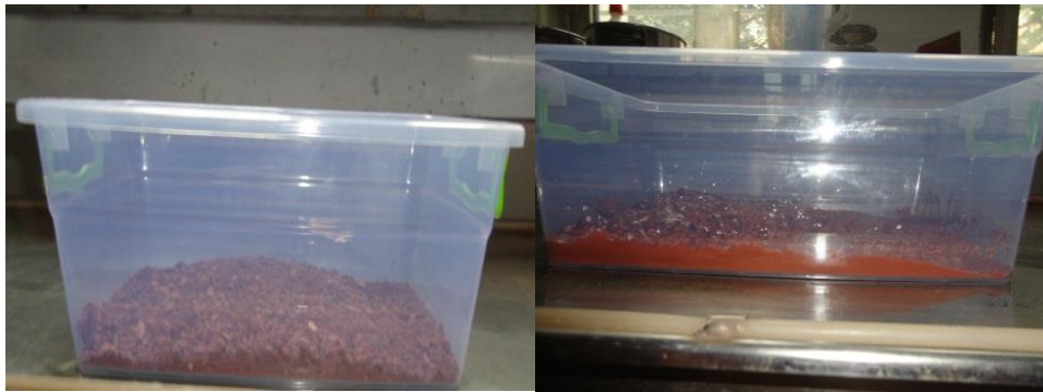
Figure 3.32 : The appearance of bauxite with different moisture content exposed to vibration after 1 hour (left-less1%), (right-10%)
