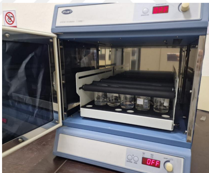
Figure 4.32 Incubator assembly for degradation testing and coating samples placed in the assembly in beakers.
