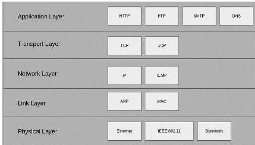
Figure 2.1: The Internet Protocol Stack with Examples for Each Layer.
