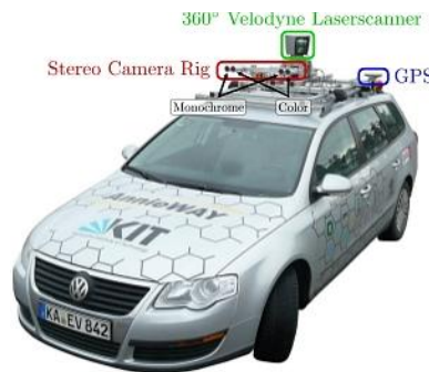
Figure 3.5. The car is used to capture KITTI sequences. It provides raw 2D stereo camera data, 3D GPS, and Velodyne Laserscanner data [45].
